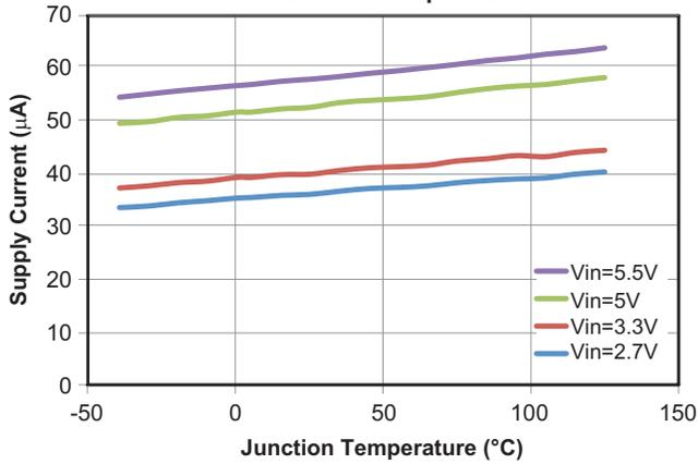
Figure 6. Supply Current, Output Disabled vs. Junction Temperature
