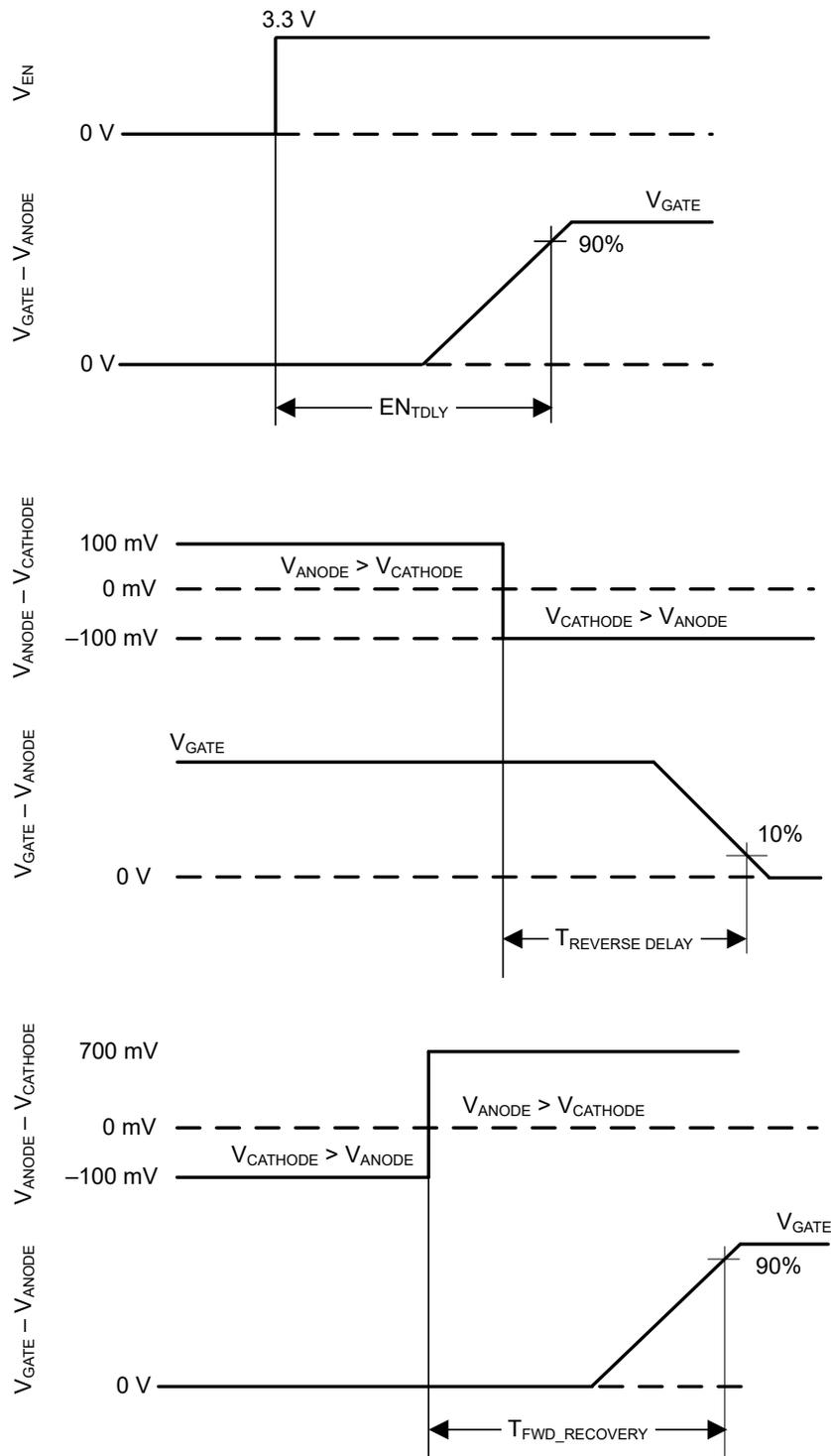
Figure 7-1. Timing Waveforms
