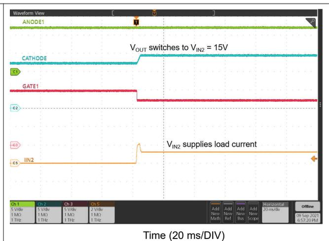
**Figure 9-14. ORing  $V_{IN1}$  to  $V_{IN2}$  Switch Over**
