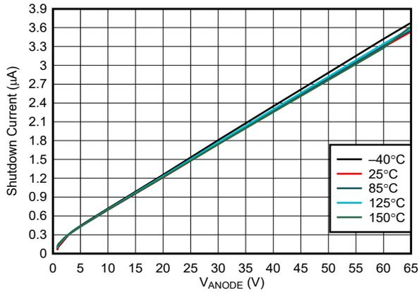
**Figure 6-1. Shutdown Supply Current vs Supply Voltage**
