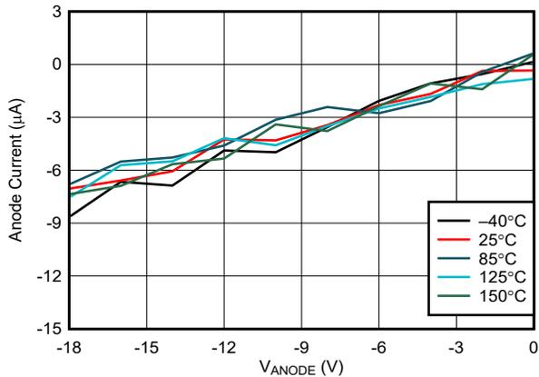
**Figure 6-3. Anode Current vs Negative Supply Voltage**
