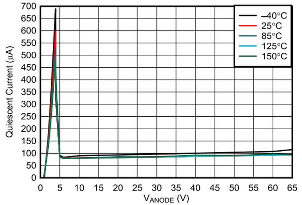
**Figure 6-2. Operating Quiescent Current vs Supply Voltage**
