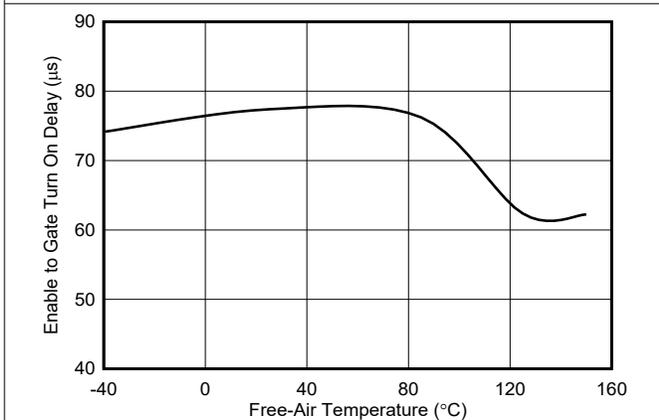
Figure 6-11. Enable to Gate Delay vs Temperature
