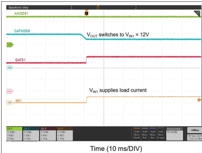
Figure 9-15. ORing  $V_{IN2}$  to  $V_{IN1}$  Switch Over
