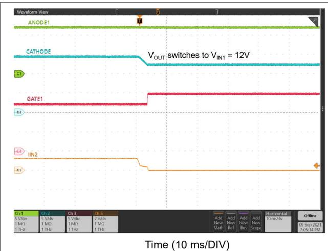
Figure 9-16. ORing  $V_{IN2}$  to  $V_{IN1}$  Switch Over
