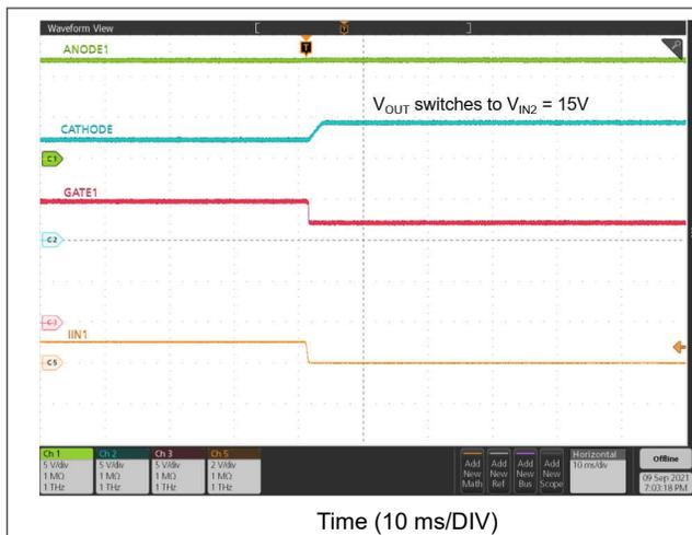
**Figure 9-13. ORing  $V_{IN1}$  to  $V_{IN2}$  Switch Over**
