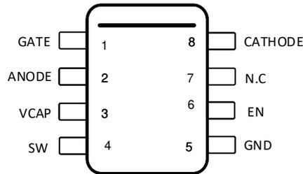
**Figure 5-1. DDF Package 8-Pin SOT-23 Top View**
