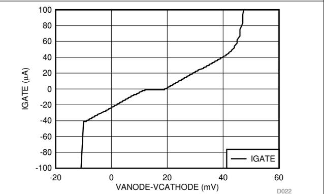
**Figure 6-16. Gate Current vs Forward Voltage Drop**
