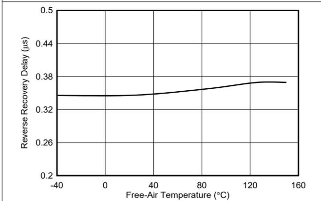
Figure 6-9. Reverse Current Blocking Delay vs Temperature
