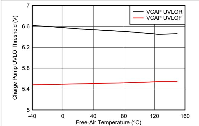
**Figure 6-13. Charge Pump UVLO Threshold vs Temperature**
