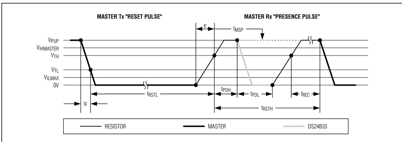
Figure 10. Initialization Procedure: Reset and Presence Pulse
