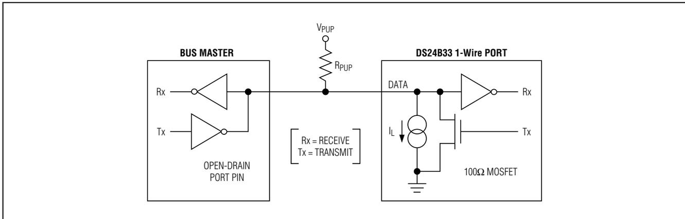
Figure 8. Hardware Configuration
