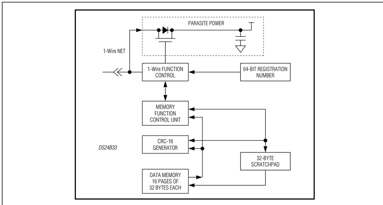
Figure 1. Block Diagram
