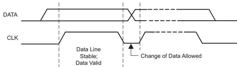
Figure 7-21. Bit Transfer on the Serial Interface
