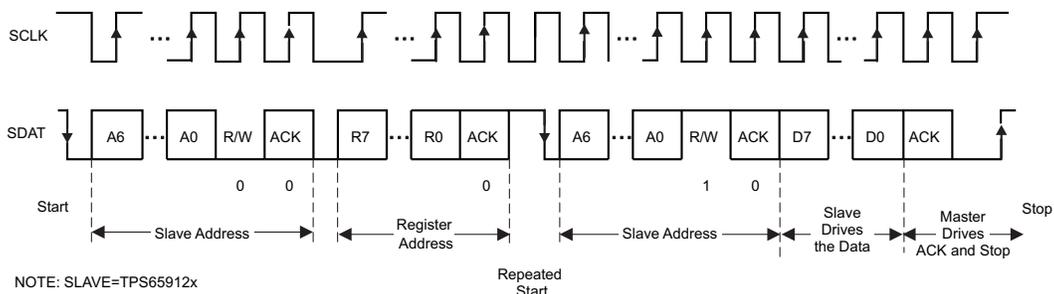
Figure 7-25. I<sup>2</sup>C Interface READ from TPS65912x; F/S mode
