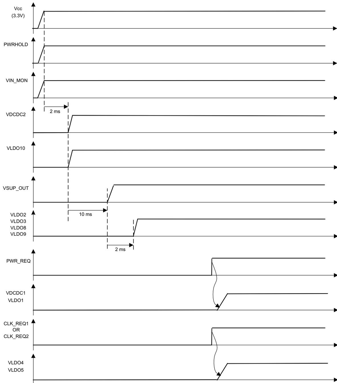
Figure 7-14. TPS659121 3.3-V Host Power Up With CONFIG1=LOW
