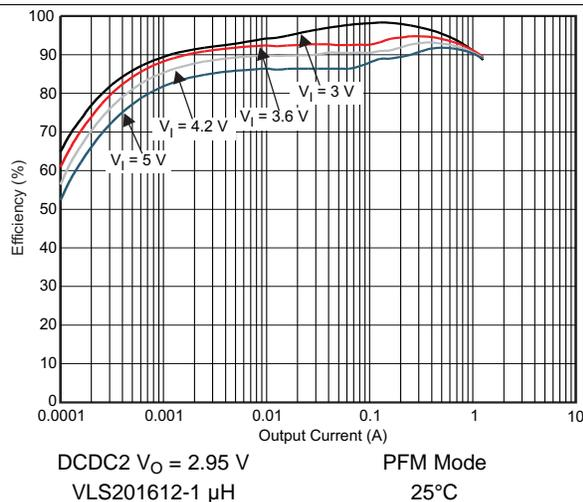
Figure 5-11. DCDC2 Efficiency vs Output Current / PFM Mode
