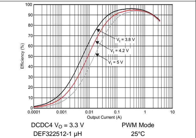
Figure 5-22. DCDC4 Efficiency vs Output Current / PWM Mode
