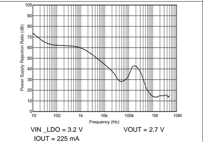
Figure 5-24. LDO4 and LDO5 PSRR vs Frequency
