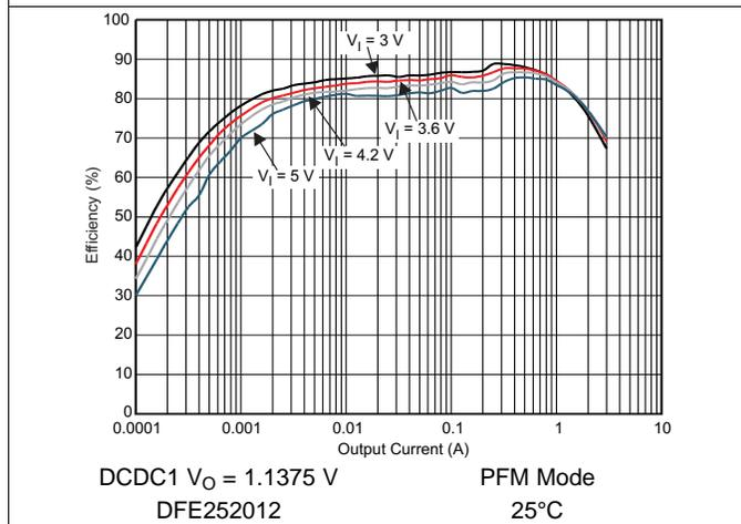
Figure 5-3. DCDC1 Efficiency vs Output Current / PFM Mode
