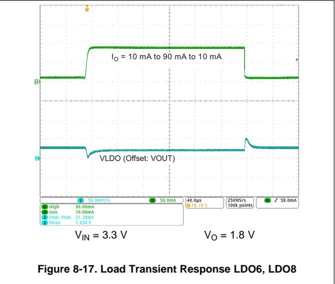
Figure 8-17. Load Transient Response LDO6, LDO8
