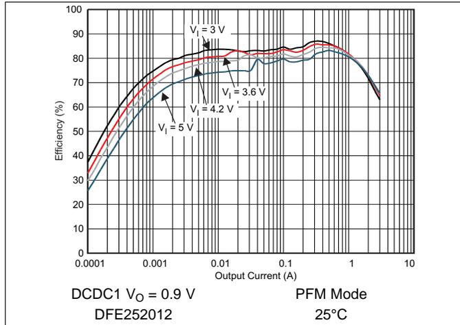
Figure 5-1. DCDC1 Efficiency vs Output Current / PFM Mode
