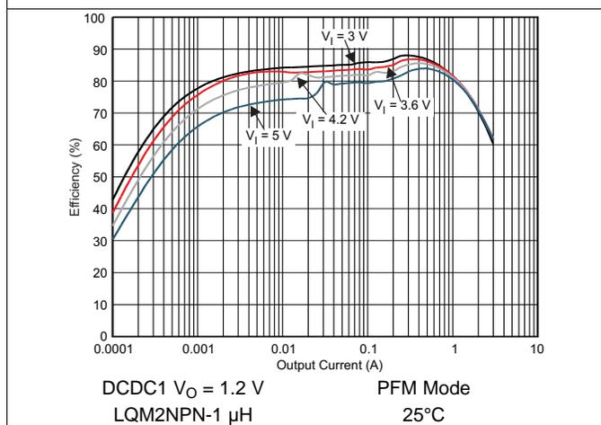
Figure 5-5. DCDC1 Efficiency vs Output Current / PFM Mode
