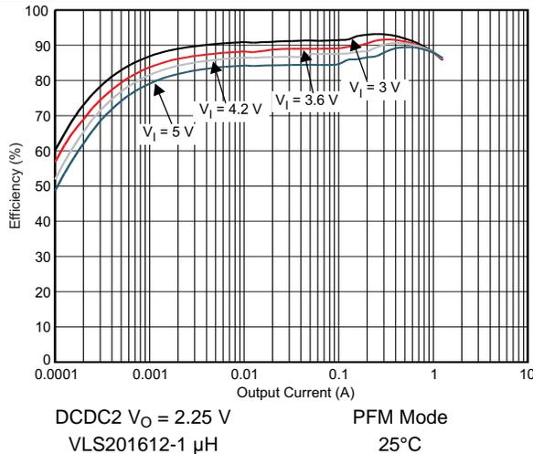
Figure 5-9. DCDC2 Efficiency vs Output Current / PFM Mode
