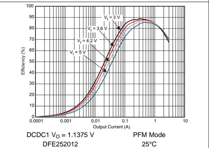
Figure 5-4. DCDC1 Efficiency vs Output Current / PWM Mode
