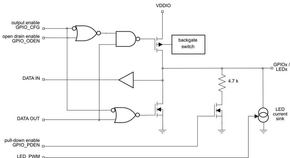
Figure 7-2. GPIO Block for GPIO3, GPIO4, and GPIO5
