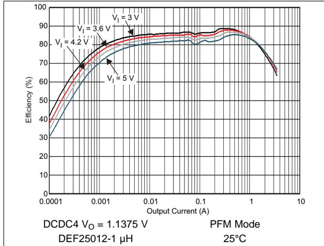
Figure 5-19. DCDC4 Efficiency vs Output Current / PFM Mode
