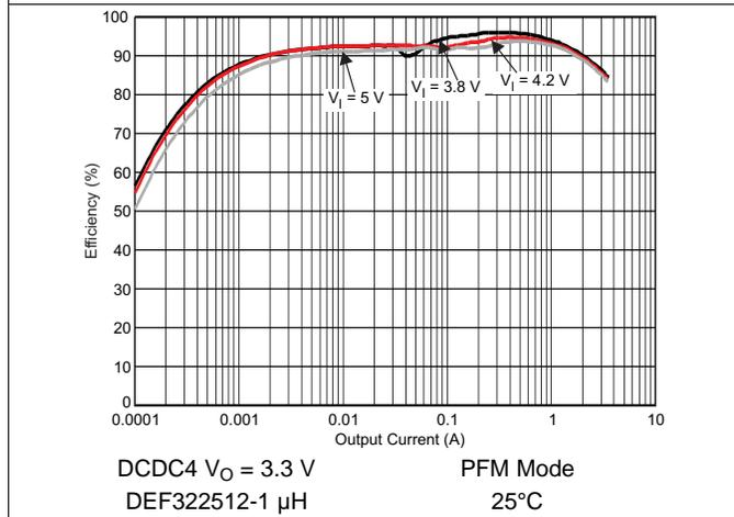
Figure 5-21. DCDC4 Efficiency vs Output Current / PFM Mode
