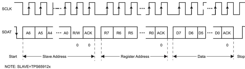
Figure 7-24. I<sup>2</sup>C Interface WRITE to TPS65912x; F/S mode
