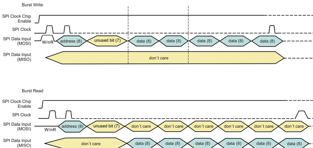
Figure 7-19. SPI BURST READ and BURST WRITE Protocol
