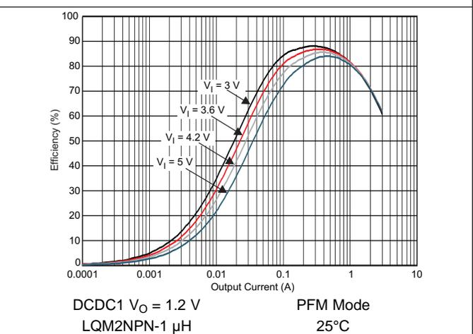
Figure 5-6. DCDC1 Efficiency vs Output Current / PWM Mode
