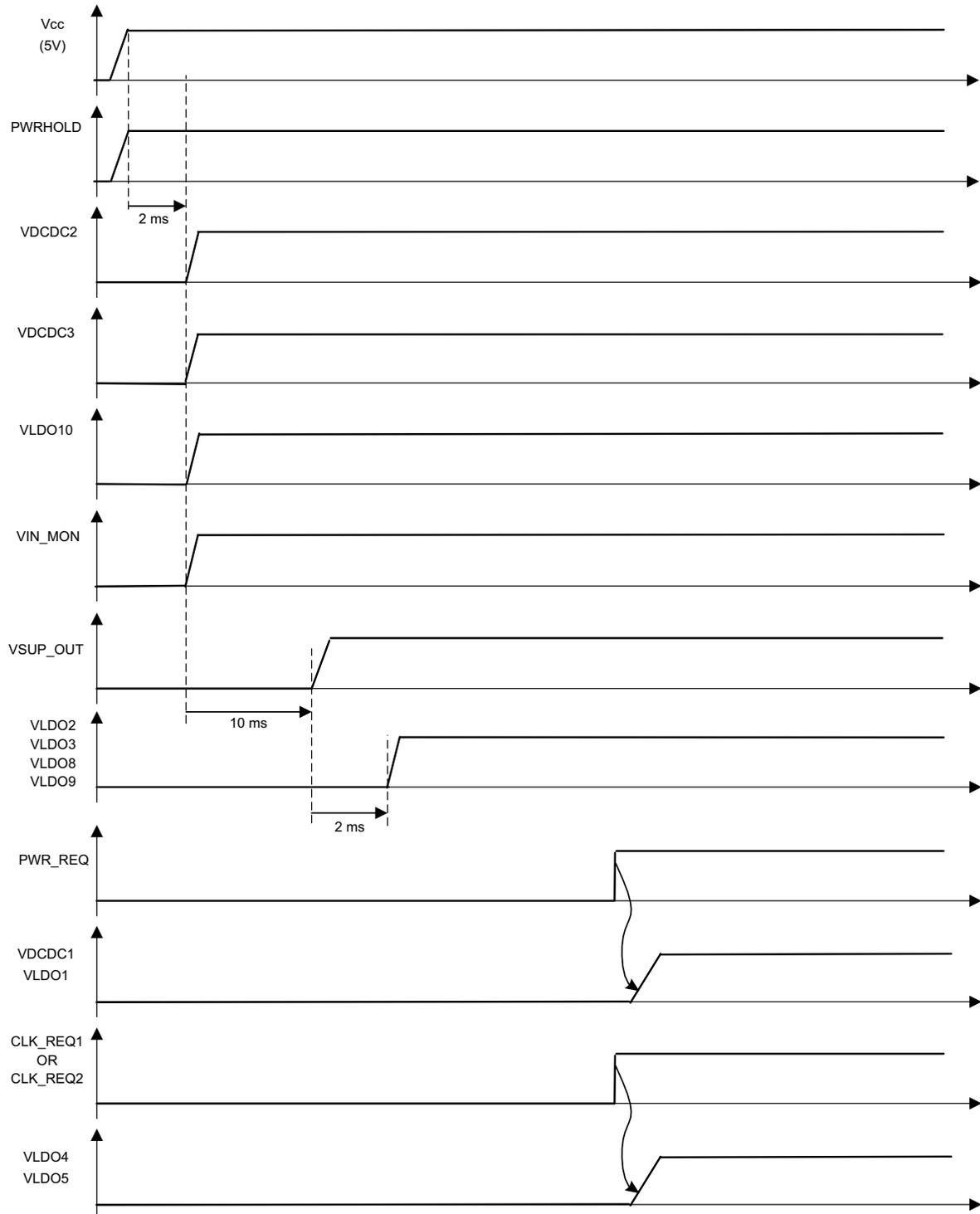
Figure 7-13. TPS659121 Battery or 5 V-USB Power-Up With CONFIG1=LOW
