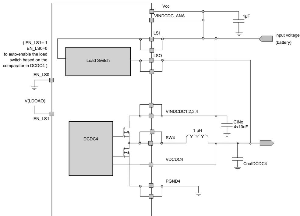
Figure 7-27. Load Switch Connected as BYPASS Switch for DCDC4
