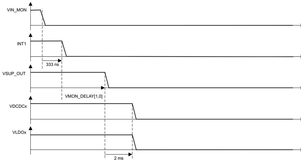
Figure 7-16. TPS659121, TPS659122 Power Cut With CONFIG1=HIGH
