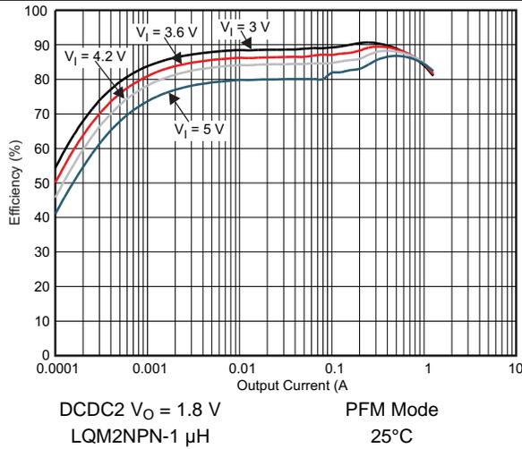
Figure 5-7. DCDC2 Efficiency vs Output Current / PFM Mode
