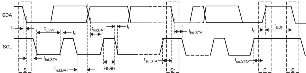
Figure 6-1. Serial Interface Timing Diagram for FS-Mode
