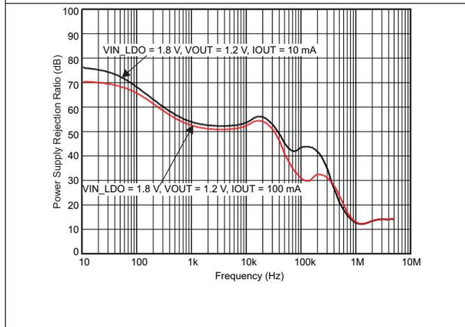
Figure 5-23. LDO1, LDO2, LDO3 PSRR vs Frequency
