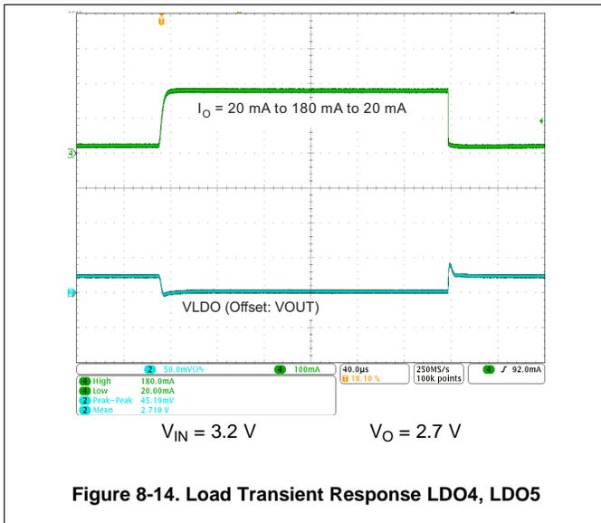
Figure 8-14. Load Transient Response LDO4, LDO5
