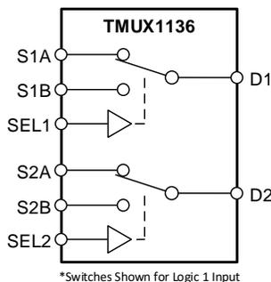
Figure 25. TMUX1136 Functional Block Diagram
