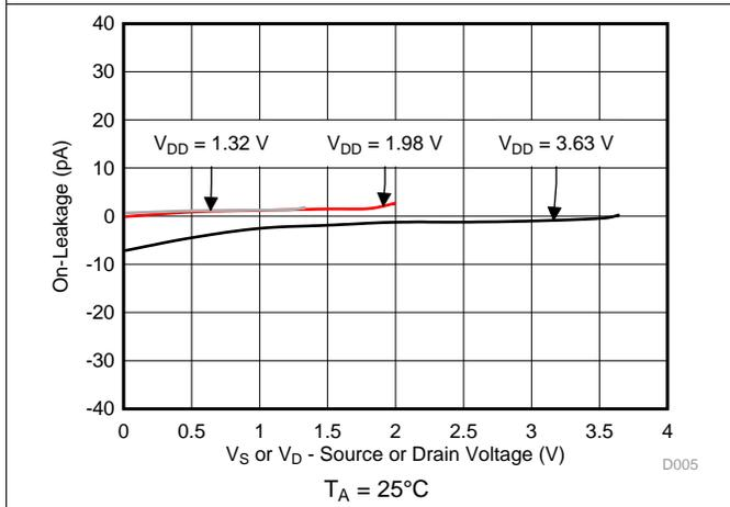
Figure 5. On-Leakage vs Source or Drain Voltage
