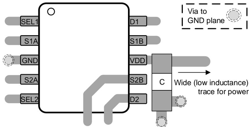
Figure 32. TMUX1136 Layout Example
