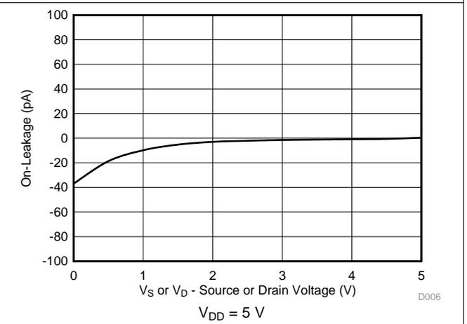
Figure 6. On-Leakage vs Source or Drain Voltage
