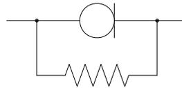
\*A 3000 $\Omega$  resistor may be added to achieve more linear regulator current characteristics.
