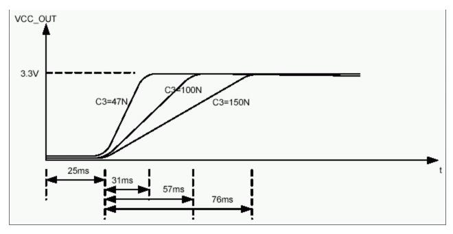
The above is response to a step-input voltage 0V to 3.3V. The current surge is well below the 360mA maximum current output with the component values given in the schematic.
