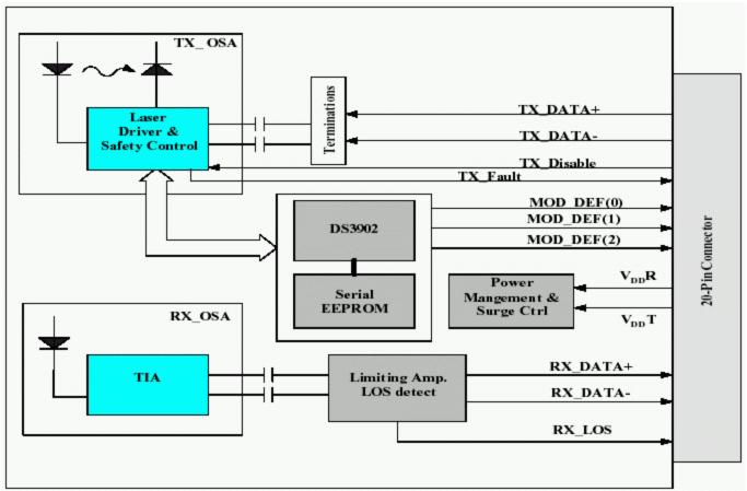
Figure 1. Typical optical module block diagram.
