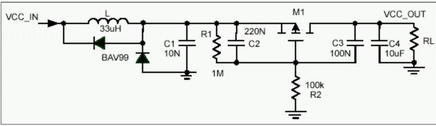
A typical slow-start circuit is depicted here. This is a low-cost design with minimum of component counts.
