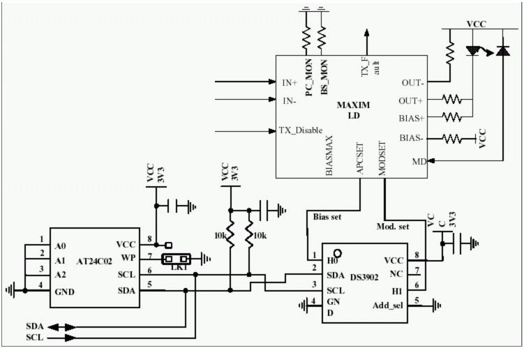
Figure 2. Schematic for LD, DS3902, and AT24C02.
