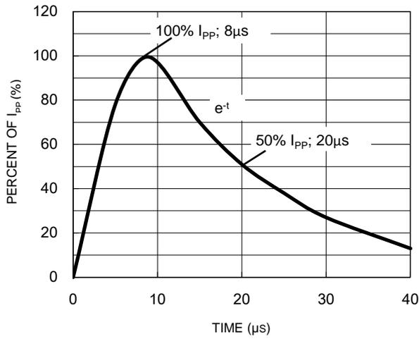
**Fig.7 ESD pulse waveform**
