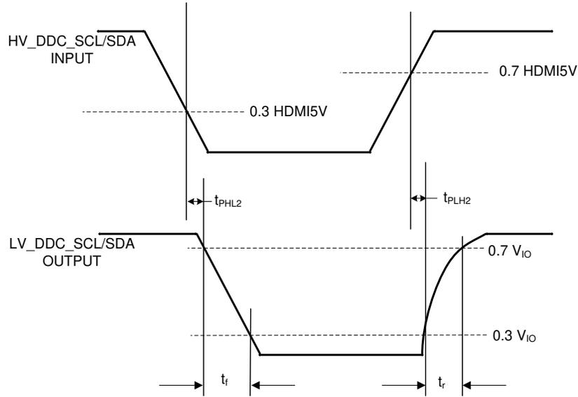
**Figure 7-11. DDC Propagation Delay – Sink to Source**
