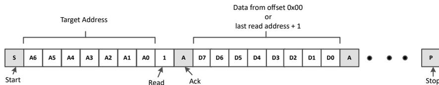
Figure 8-12. I<sup>2</sup>C Read Without Repeated Start
