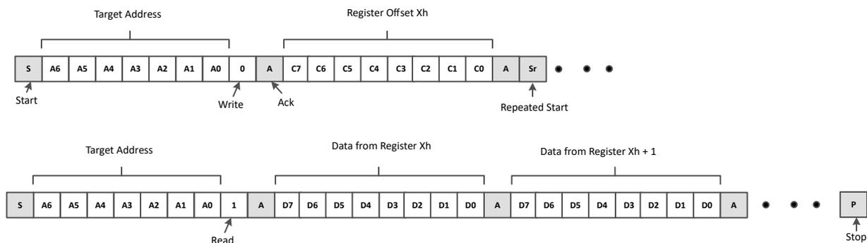
Figure 8-13. I<sup>2</sup>C Read with Repeated Start
