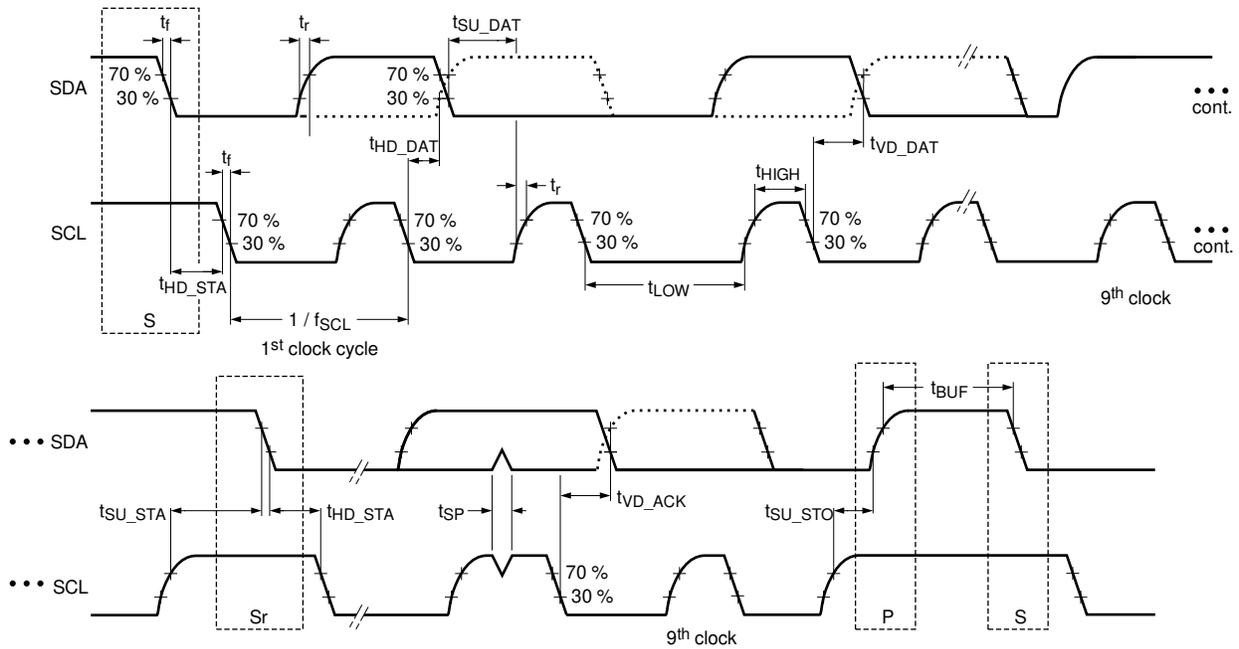
**Figure 7-9. I<sup>2</sup>C SCL and SDA Timing**
