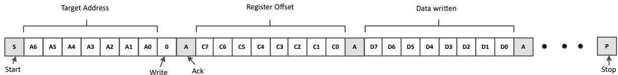
Figure 8-11. I<sup>2</sup>C Write with Data
