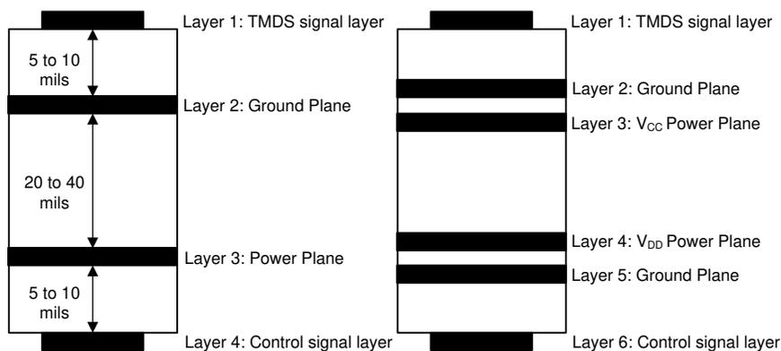
**Figure 11-1. Recommended 4 or 6-Layer PCB Stack**
