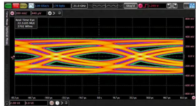
**Figure 9-6. 12 Gbps Input Eye at TTP2 After Pre-channel**
