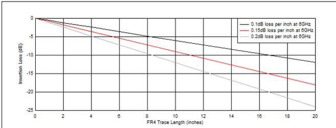
**Figure 9-3. FR4 Trace Insertion Loss at 6 GHz**
