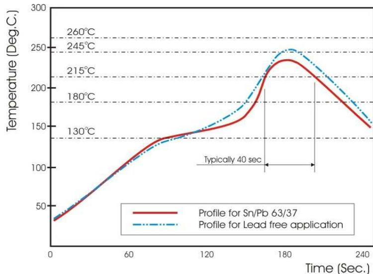
**Fig 3. Infrared soldering profile for Chip Resistors WFxxS**
