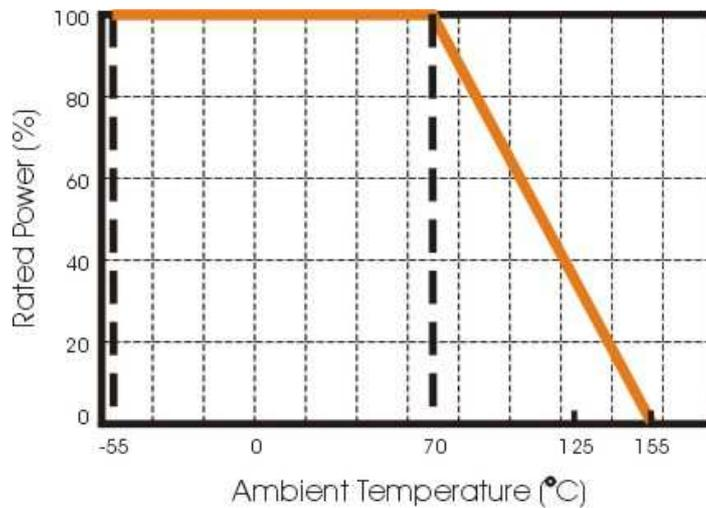
Fig.2 Maximum dissipation in percentage of rated power
