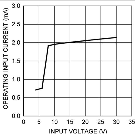
Figure 8. Operating Input Current vs Input Voltage
