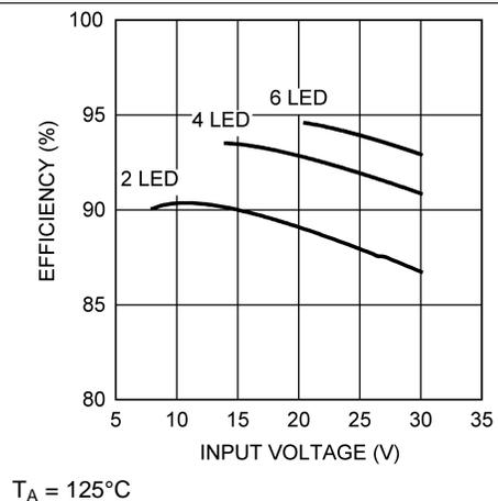
Figure 6. Efficiency vs Input Voltage
