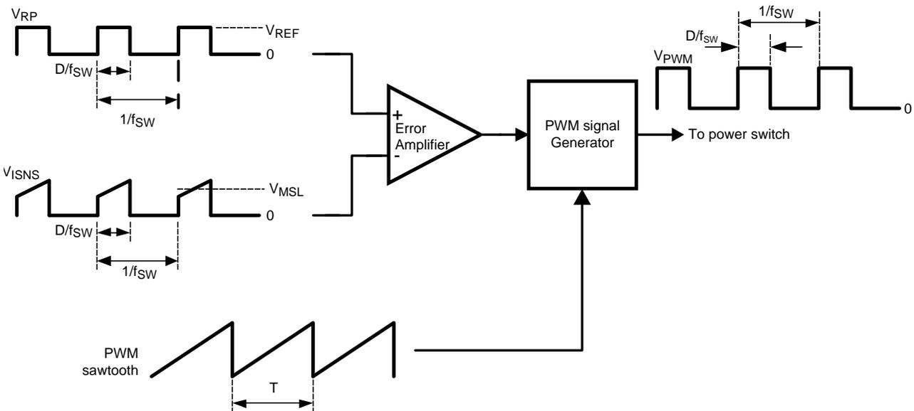
**Figure 21. Implementation of the PWM Switching Signal**
