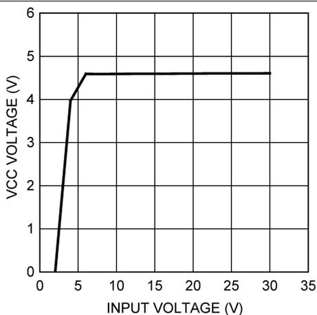
Figure 9. VCC Voltage vs Input Voltage
