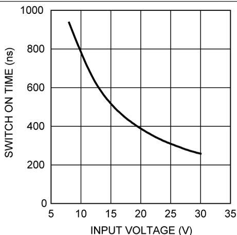
Figure 7. Switch On Time vs Input Voltage
