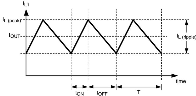
Figure 23. Relationship Between  $I_{OUT}$ ,  $I_{L(peak)}$  and  $I_{L(ripple)}$
