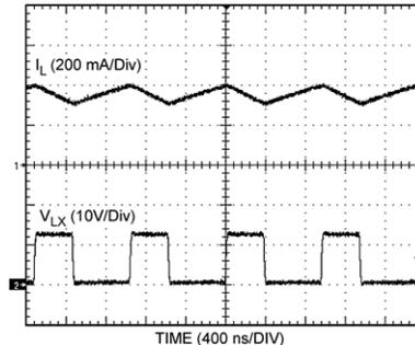
Figure 25. LED Current and Switch Voltage Waveforms
