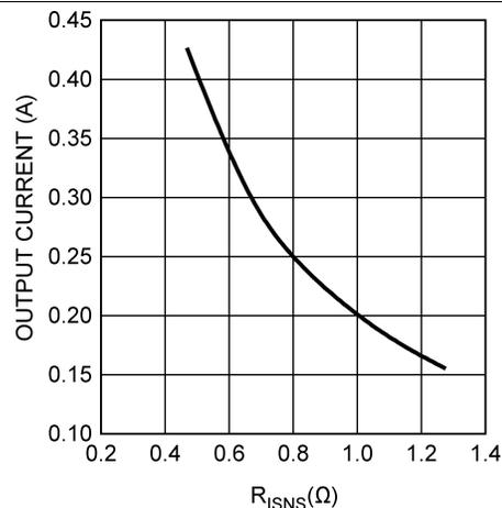
Figure 10. Output Current vs R\_ISNS
