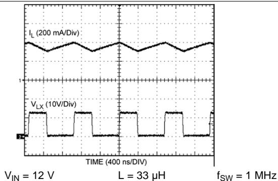
Figure 12. Continuous Mode Operation
