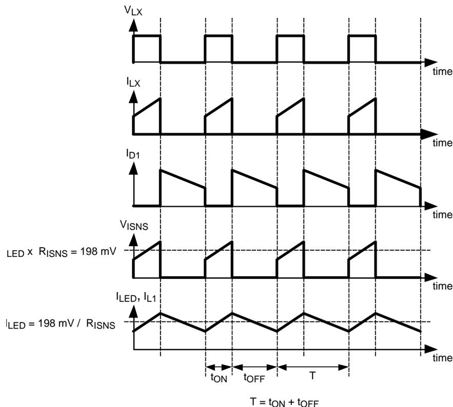
**Figure 18. Operating Waveforms of a Floating Buck Converter**
