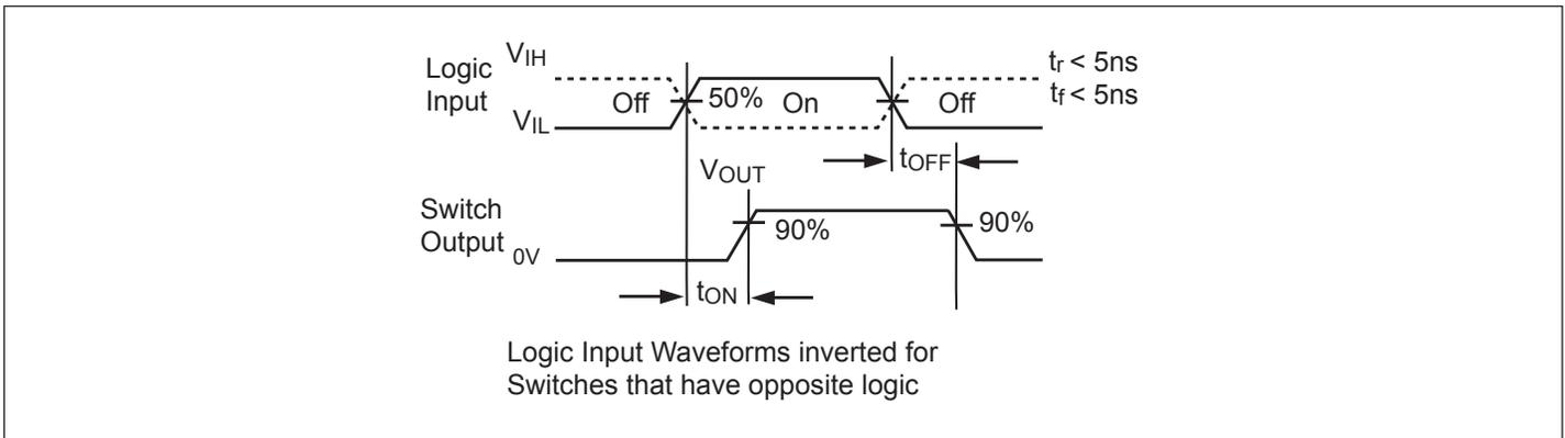
**Figure 2. AC Waveforms**
