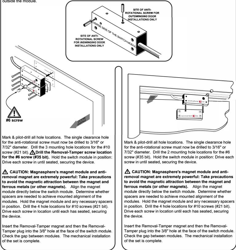
\*\*Recommended placement to meet door opening and alarm requirements of UL634 Level 2. This guide is one means to meet this standard. Installations which fulfill its requirements are not restricted to the specific recommendations in this instruction set.
