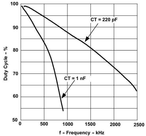
**Figure 7-18. Maximum Duty Cycle vs Oscillator Frequency**
