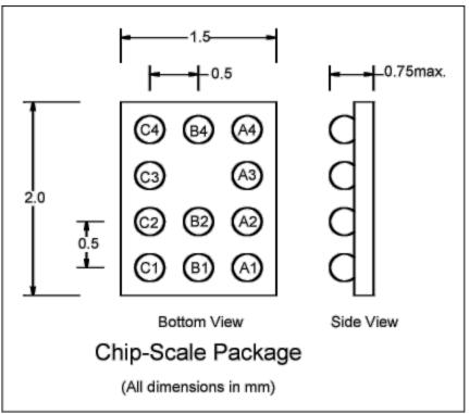
Figure 9. Ultra-chip-scale package.
