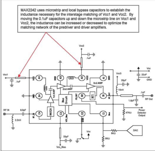
Figure 2. MAX2242 application circuit.
