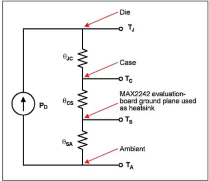
Figure 8. Electrical equivalent circuit of the thermal-conduction process.
