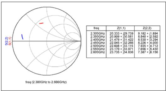
Figure 5. Optimum source and load impedance.
