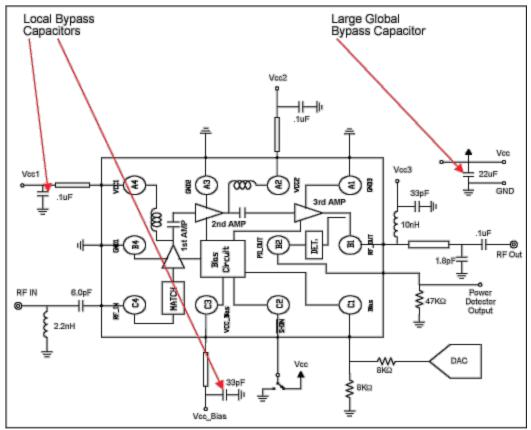
Figure 6. Application schematic with internal block diagram.
