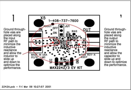
Figure 1. Top-component view of the MAX2242 evaluation board.
