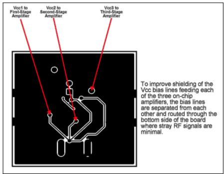
Figure 7. Bottom-side view of the MAX2242 evaluation board.
