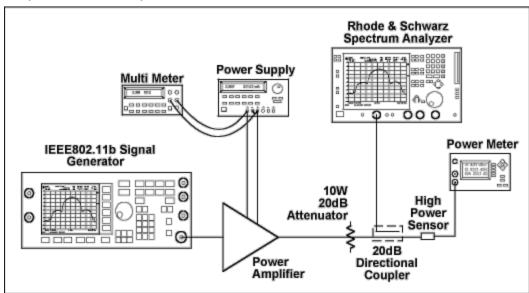
Figure 10. MAX2242 test setup.
