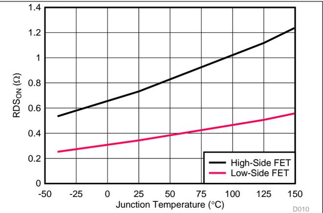
Figure 8. MOSFETs On-State Resistance vs Temperature D010
