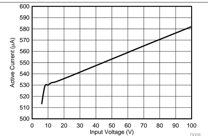
Figure 6.  $V_{IN}$  Active Current vs Input Voltage
