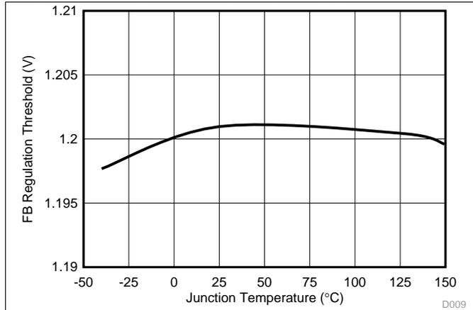
Figure 7. Feedback Comparator Threshold vs Temperature D009
