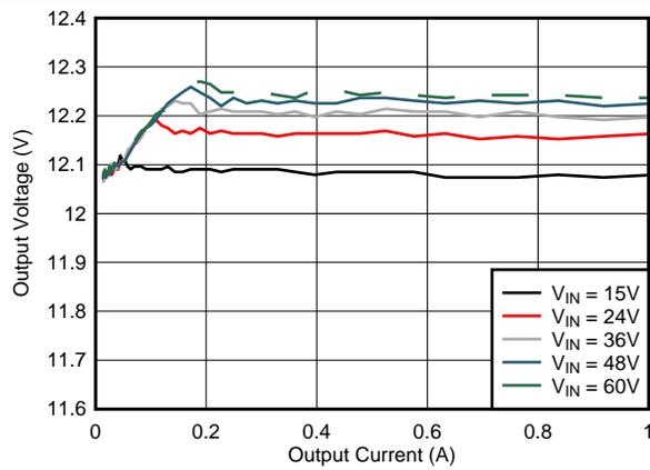
Figure 15. Load and Line Regulation Performance
