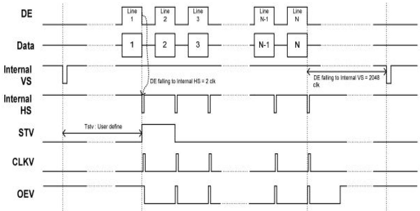
8.6 Input Data Timing (24 bit RGB mode for 960 x 240 @ SEL[3:0] = 1100b)
