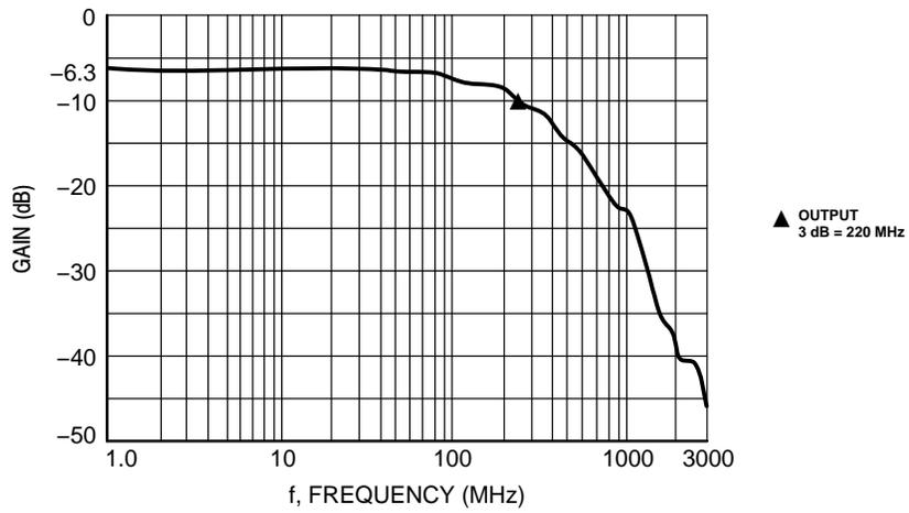
Figure 2. Typical EMI Filter Response
