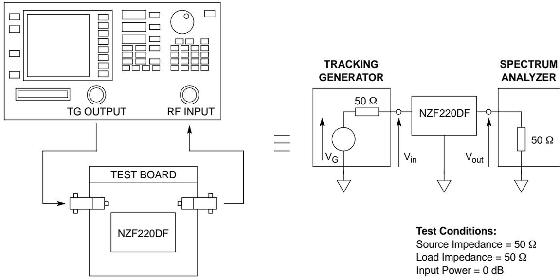
Figure 1. Measurement Conditions
