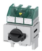
SENTRON, Molded case switch 3LD5 UL, Main switch, 3-pole, certified according to UL489 UL60947-4-1 and IEC60947-3, UL: 30A, SCCR 50kA at 480VAC, Operating power at 480VAC 3-phase: 20hp, IEC: 32A, Operating power at AC-23A at 400V: 15kW, floor mounting with direct handle, black, incl. terminal covers for the infeed side
