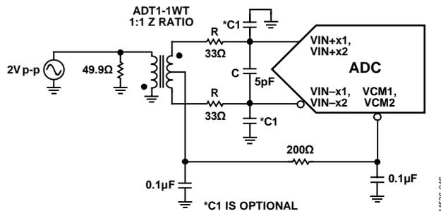
Figure 36. Differential Transformer Coupled Configuration for Baseband Applications
