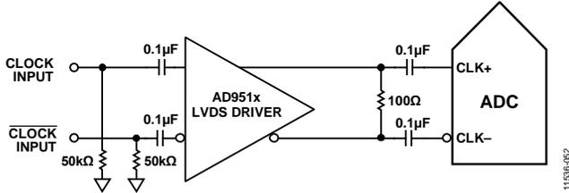
Figure 42. Differential LVDS Sample Clock (Up to 520 MHz)
