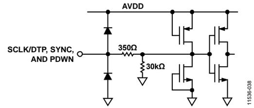
Figure 28. Equivalent SCLK/DTP, SYNC, and PDWN Input Circuit
