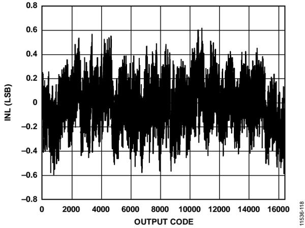
Figure 19. INL;  $f_{IN} = 9.7 \text{ MHz}$ ,  $f_{SAMPLE} = 65 \text{ MSPS}$
