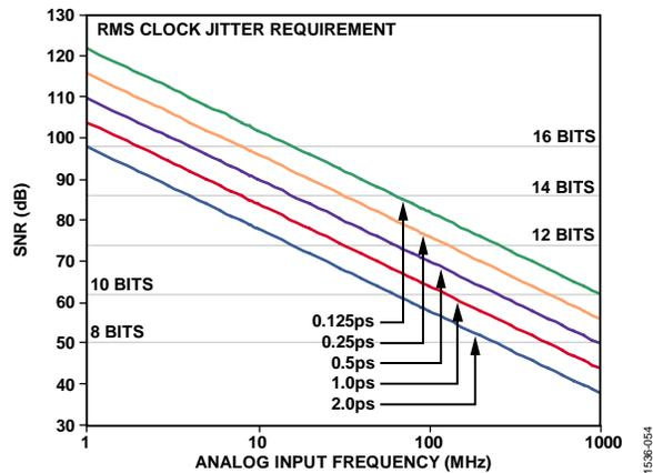
Figure 44. Ideal SNR vs. Input Frequency and Jitter
