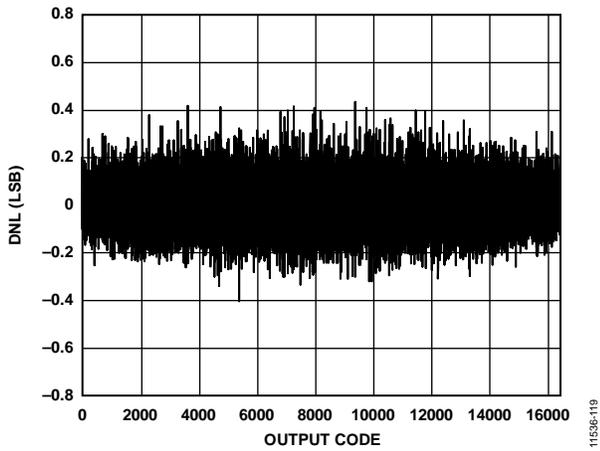
Figure 20. DNL;  $f_{IN} = 9.7 \text{ MHz}$ ,  $f_{SAMPLE} = 65 \text{ MSPS}$
