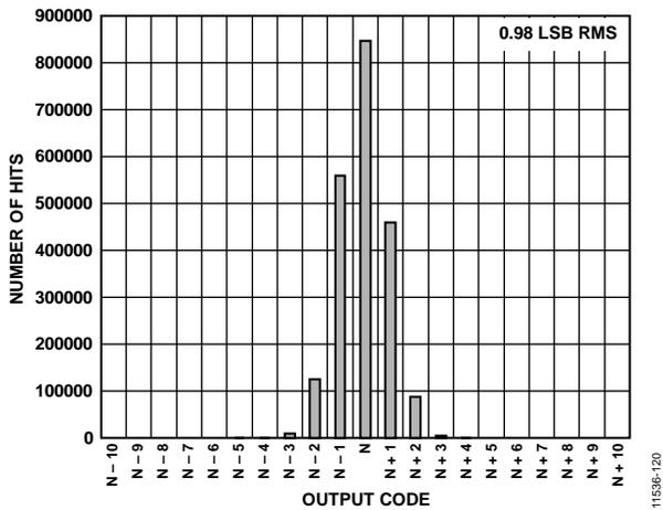
Figure 21. Input Referred Noise Histogram;  $f_{SAMPLE} = 65 \text{ MSPS}$
