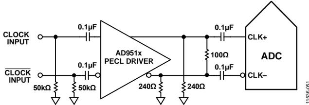
Figure 41. Differential PECL Sample Clock (Up to 520 MHz)
