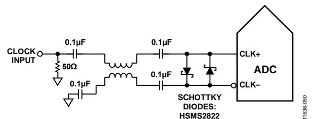
Figure 40. Balun-Coupled Differential Clock (65 MHz to 520 MHz)
