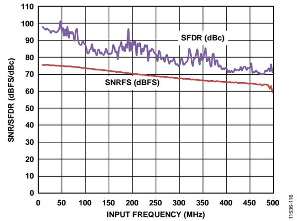
Figure 17. SNR/SFDR vs.  $f_{IN}$ ;  $f_{SAMPLE} = 65$  MSPS
