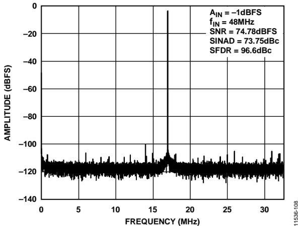
Figure 9. Single-Tone 32k FFT with  $f_{IN} = 48\text{ MHz}$ ,  $f_{SAMPLE} = 65\text{ MSPS}$
