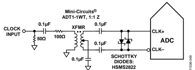
Figure 39. Transformer-Coupled Differential Clock (Up to 200 MHz)
