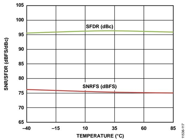
Figure 18. SNR/SFDR vs. Temperature;  $f_{IN} = 9.7$  MHz,  $f_{SAMPLE} = 65$  MSPS
