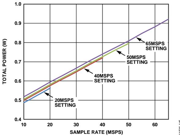
Figure 45. Total Power vs.  $f_{SAMPLE}$  for  $f_{IN} = 9.7$  MHz
