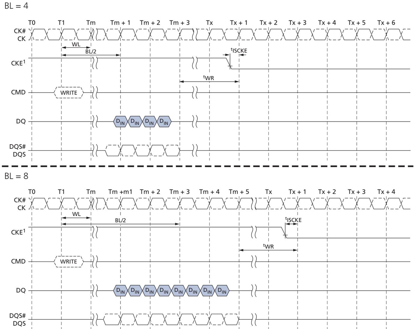
Note: 1. CKE can be registered LOW at  $(WL + 1 + BL/2 + RU(tWR/tCK))$  clock cycles after the clock on which the WRITE command is registered.
