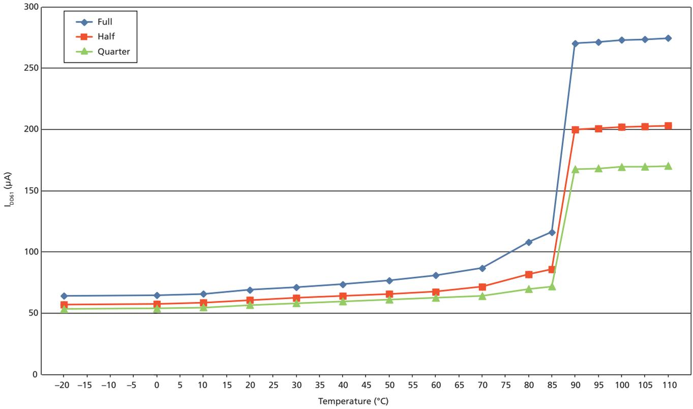
Figure 3: I<sub>DD62</sub> Typical Self Refresh Current vs. Temperature
