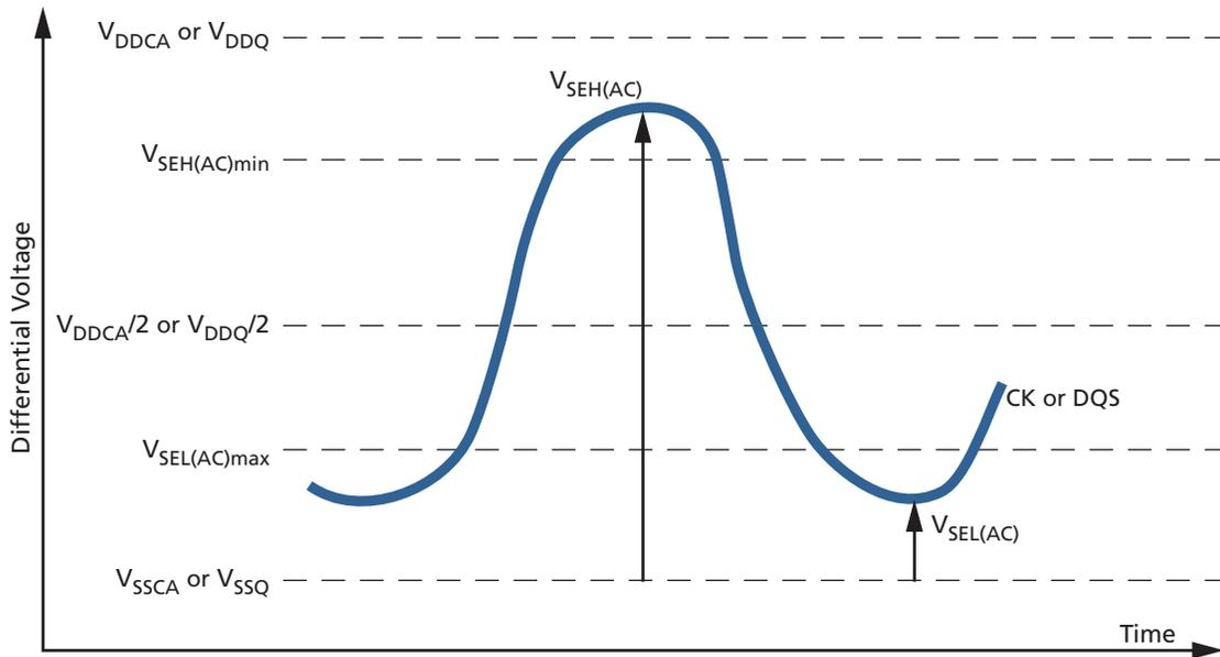
Note that while CA and DQ signal requirements are referenced to  $V_{REF}$ , the single-ended components of differential signals also have a requirement with respect to  $V_{DDQ}/2$  for DQS, and  $V_{DDCA}/2$  for CK.
