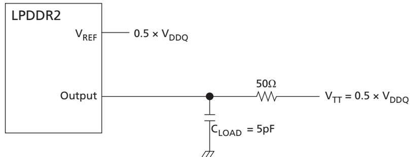
Note: 1. All output timing parameter values ( $t_{DQSCK}$ ,  $t_{DQSQ}$ ,  $t_{QHS}$ ,  $t_{HZ}$ ,  $t_{RPRE}$  etc.) are reported with respect to this reference load. This reference load is also used to report slew rate.
