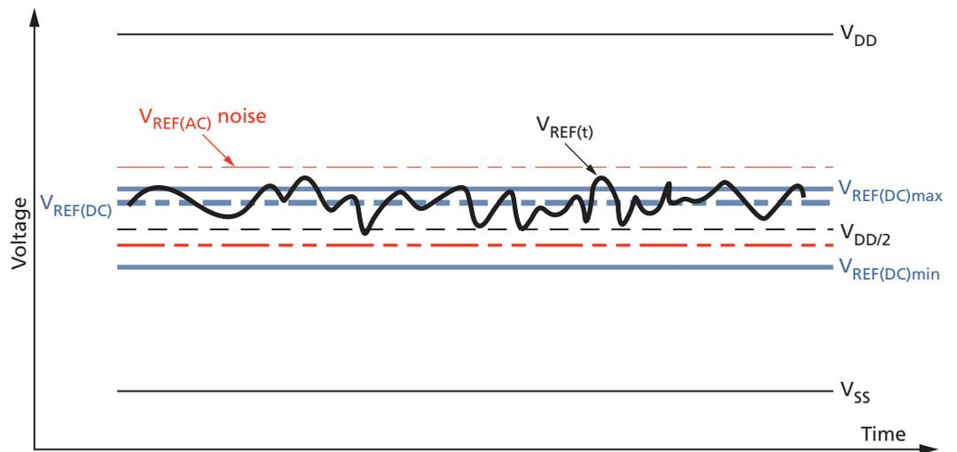
The voltage levels for setup and hold time measurements V<sub>IH(AC)</sub>, V<sub>IH(DC)</sub>, V<sub>IL(AC)</sub>, and V<sub>IL(DC)</sub> are dependent on V<sub>REF</sub>.
