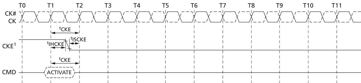
Note: 1. CKE can go LOW at  $t_{IHCKE}$  after the clock on which the ACTIVATE command is registered.
