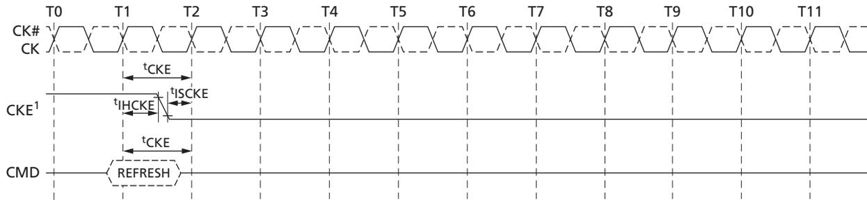
Note: 1. CKE can go LOW  $t_{IHCKE}$  after the clock on which the REFRESH command is registered.
