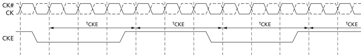
Figure 54: REFRESH-to-REFRESH Timing in CKE Intensive Environments
