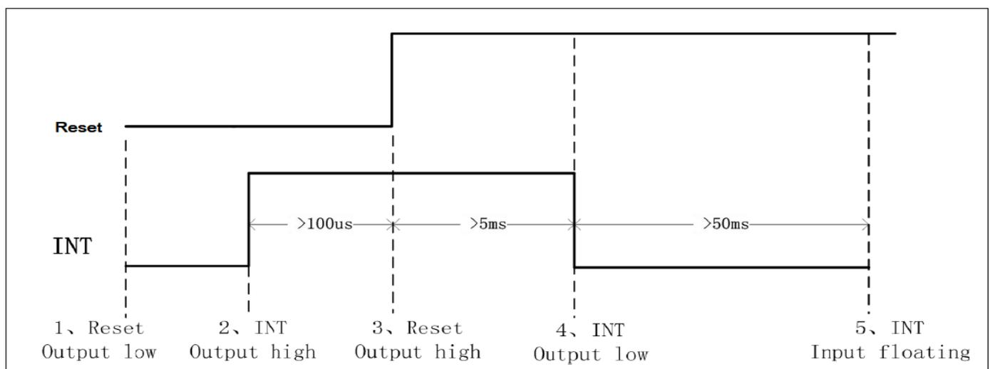
**Figure 7.3: Setting Slave Address to 0x28/0x29 Timing**
