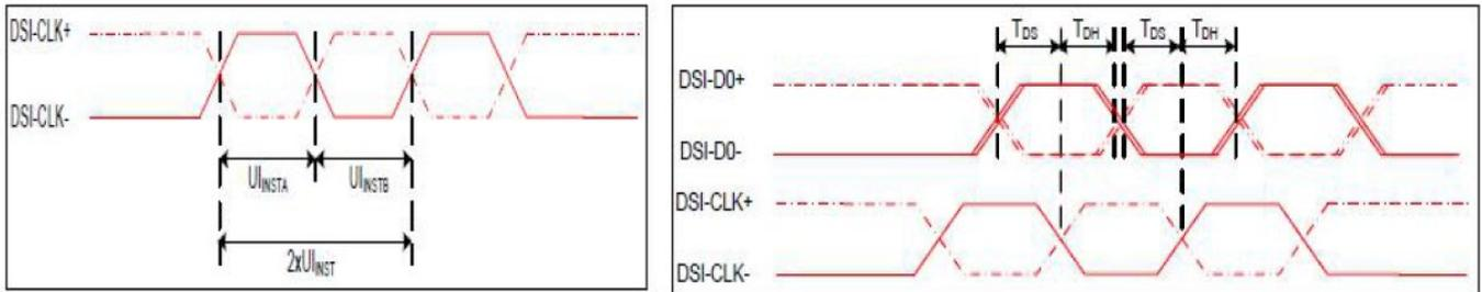
Figure 6.1: DSI Clock Channel Timing Diagram
