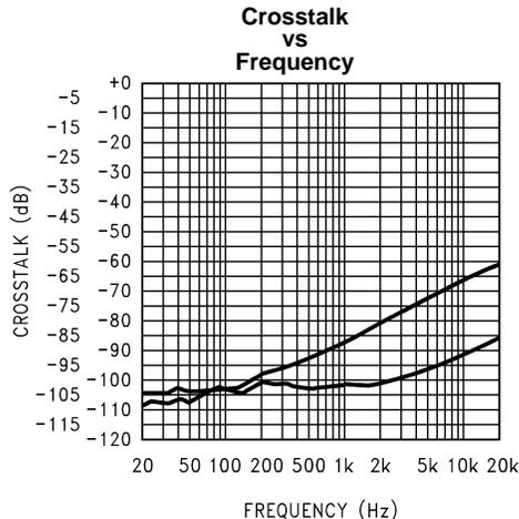
Figure 32.  $V_{DD} = 5V$ ; LLS, RLS;  $P_O = 400mW$ ;  $R_L = 8\Omega$ ; Mode 7; 0db Gain; 3D off
