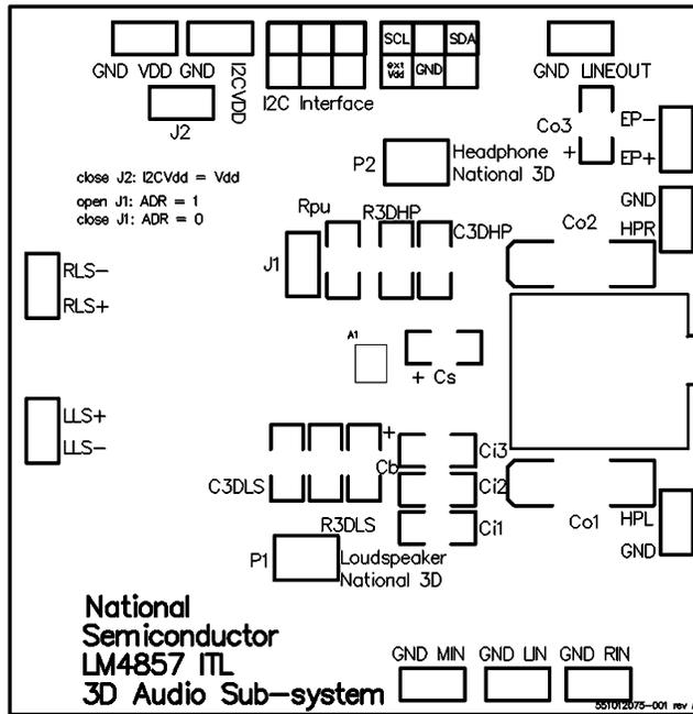
**Figure 56. Recommended DSBGA PCB Layout:
