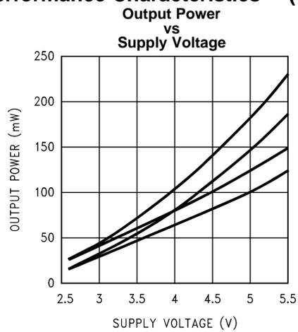
**Figure 52. EP;  $R_L = 32\Omega$ ;**
