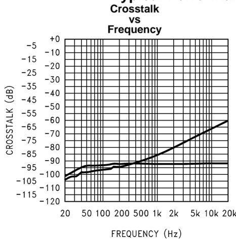
Figure 34.  $V_{DD} = 5V$ ; LHP, RHP;  $P_O = 15mW$ ;  $R_L = 32\Omega$ ; Mode 9; 0db Gain; 3D off
