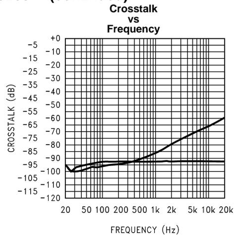
Figure 35.  $V_{DD} = 3V$ ; LHP, RHP;  $P_O = 10mW$ ;  $R_L = 32\Omega$ ; Mode 9; 0db Gain; 3D off
