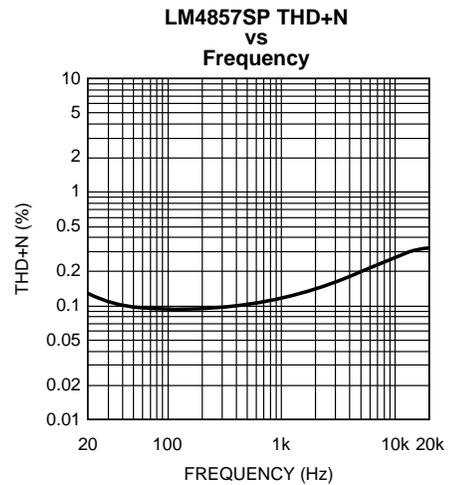
Figure 5.  $V_{DD} = 3V$ ; LLS, RLS;  $P_O = 200mW$ ;  $R_L = 4\Omega$ ; Mode 7; 0dB Gain
