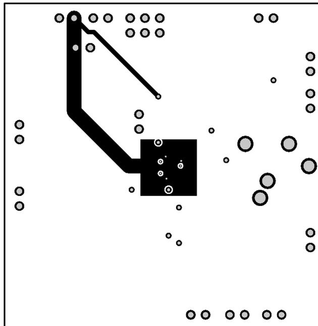
Figure 59. Recommended DSBGA PCB Layout:
