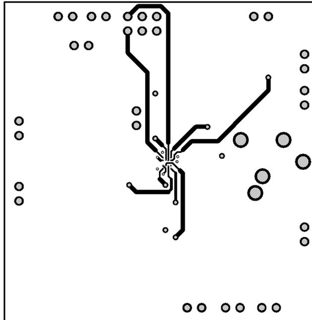
Figure 58. Recommended DSBGA PCB Layout:
