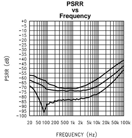
Figure 31.  $V_{DD} = 3V$ ; LINEOUT;  $R_L = 5k\Omega$ ; 0db Gain; All audio inputs terminated
