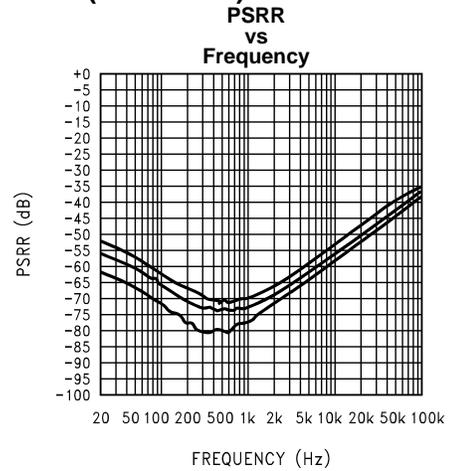
Figure 29.  $V_{DD} = 3V$ ; EP;  $R_L = 32\Omega$ ; 0db Gain; All audio inputs terminated
