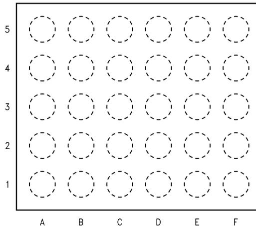
Figure 2. 30 Bump DSBGA Package – Top View (Bump-side down)
