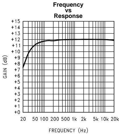
Figure 42. LINEOUT;  $R_L = 5k\Omega$ ;  $C_O = 2.2\mu F$
