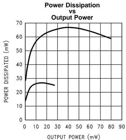
Figure 44. LHP, RHP;  $R_L = 32\Omega$ ; THD+N  $\leq 1\%$
