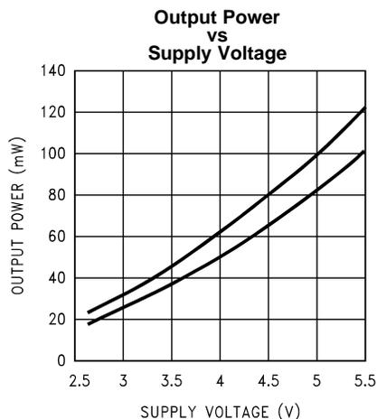
**Figure 51.** LHP, RHP;  $R_L = 32\Omega$ ;
