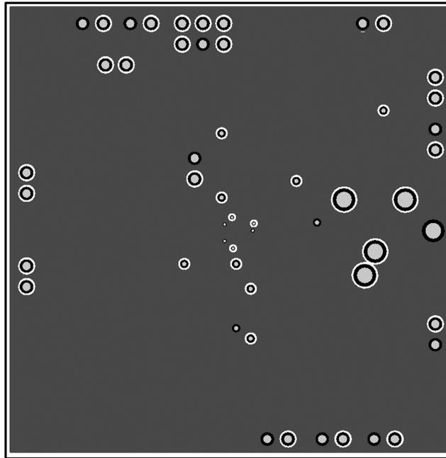
Figure 60. Recommended DSBGA PCB Layout: Bottom Layer
