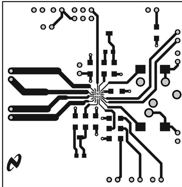
**Figure 57. Recommended DSBGA PCB Layout:
