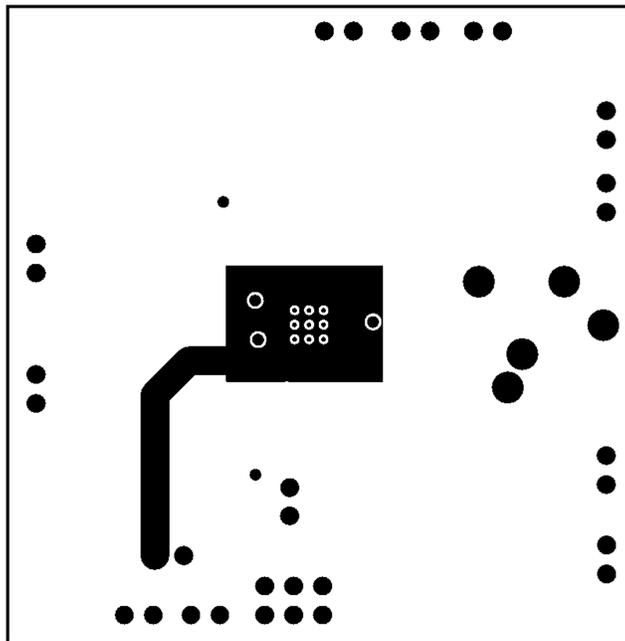
Figure 63. Recommended UQFN PCB Layout:
