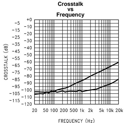
Figure 33.  $V_{DD} = 3V$ ; LLS, RLS;  $P_O = 200mW$ ;  $R_L = 8\Omega$ ; Mode 7; 0db Gain; 3D off
