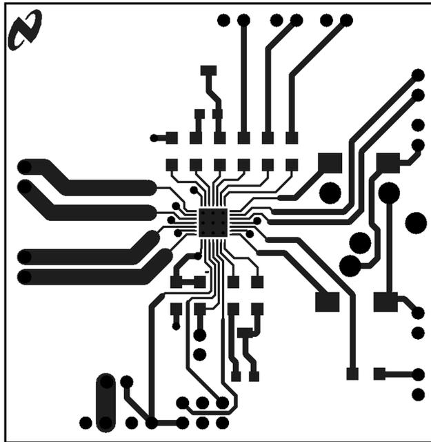
Figure 62. Recommended UQFN PCB Layout:
