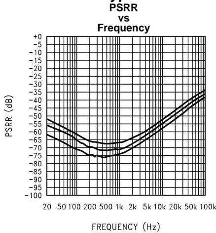
Figure 28.  $V_{DD} = 5V$ ; EP;  $R_L = 32\Omega$ ; 0db Gain; All audio inputs terminated
