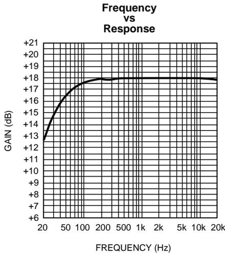
Figure 36. LLS, RLS;  $R_L = 8\Omega$ ; Mode 2; Full Gain
