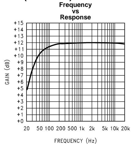
Figure 41. LINEOUT;  $R_L = 5k\Omega$ ;  $C_O = 2.2\mu F$
