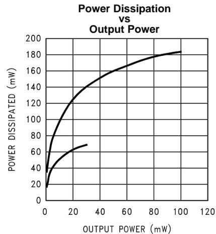
Figure 45. EP;  $R_L = 32\Omega$ ; THD+N  $\leq 1\%$
