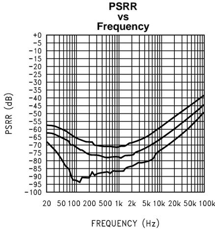
Figure 30.  $V_{DD} = 5V$ ; LINEOUT;  $R_L = 5k\Omega$ ; 0db Gain; All audio inputs terminated
