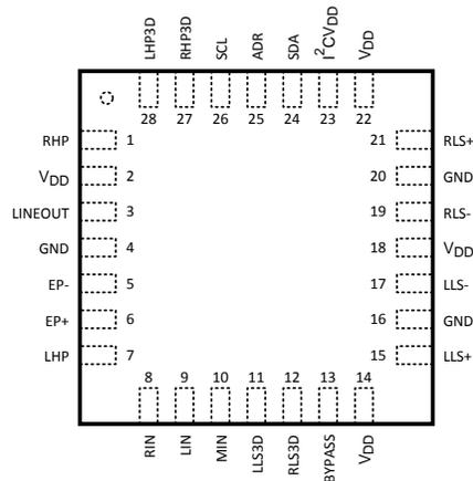
**Figure 3. 28 – UQFN Package, Top View**
