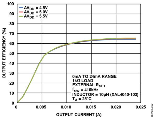
Figure 58. Output Efficiency vs. Output Current (See Figure 81)
