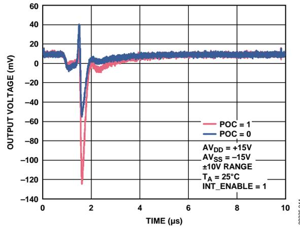
Figure 31.  $V_{OUT\_x}$  vs. Time on Output Enable
