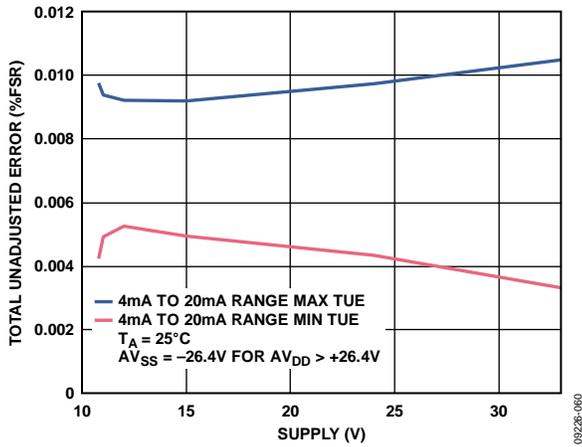
Figure 46. Total Unadjusted Error vs.  $AV_{DD}$ , External  $R_{SET}$
