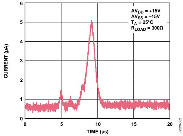
Figure 48. Output Current vs. Time on Power-Up
