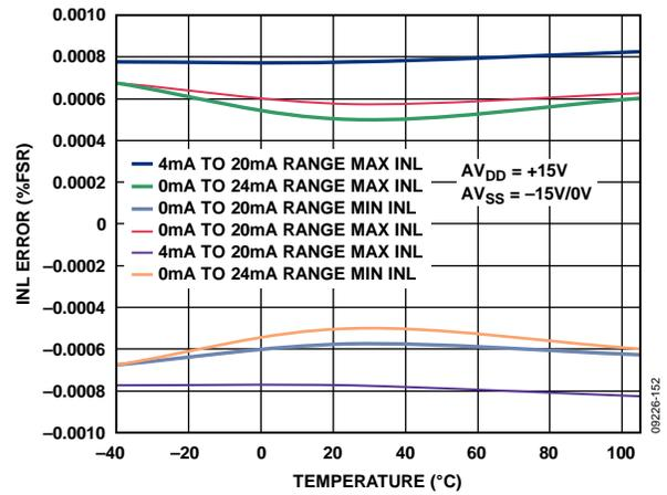
Figure 36. Integral Nonlinearity vs. Temperature, Internal RSET
