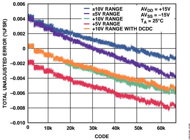
Figure 11. Total Unadjusted Error vs. DAC Code
