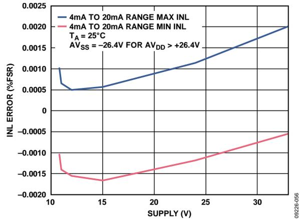
Figure 43. Integral Nonlinearity Error vs. AV<sub>DD</sub>/|AV<sub>SS</sub>| Over Supply, External R<sub>SET</sub>
