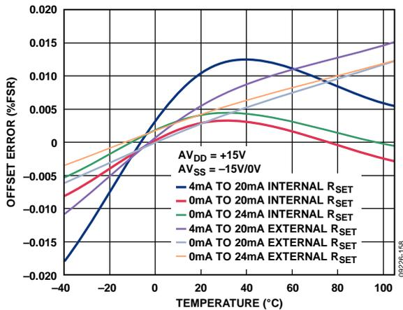
Figure 41. Offset Error vs. Temperature
