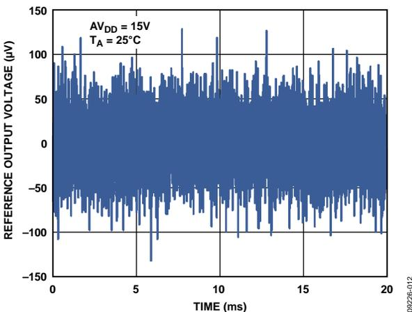
Figure 63. REFOUT Output Noise (100 kHz Bandwidth)
