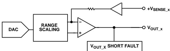
Figure 73. Voltage Output
