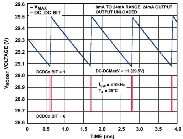
Figure 82. Operation on Reaching V<sub>MAX</sub>
