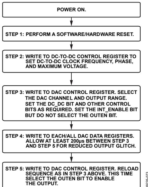
Figure 76. Programming Sequence for Enabling the Output Correctly
