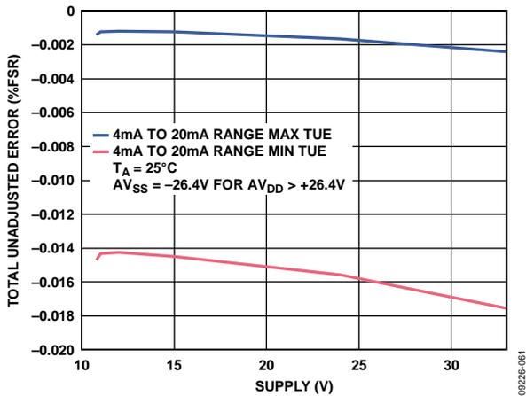
Figure 47. Total Unadjusted Error vs.  $AV_{DD}$ , Internal  $R_{SET}$
