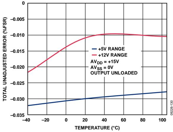
Figure 15. Total Unadjusted Error vs. Temperature, Single Supply
