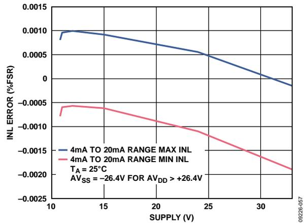
Figure 44. Integral Nonlinearity Error vs. AV<sub>DD</sub>/|AV<sub>SS</sub>| Over Supply, Internal R<sub>SET</sub>
