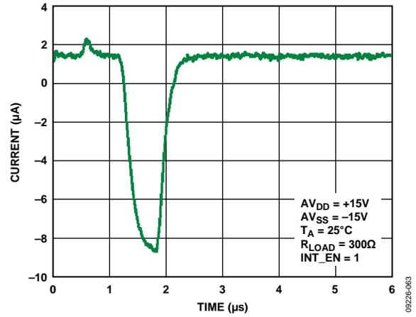
Figure 49. Output Current vs. Time on Output Enable
