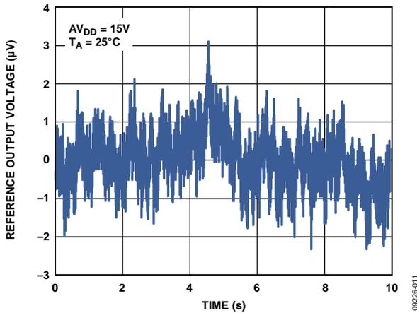
Figure 62. REFOUT Output Noise (0.1 Hz to 10 Hz Bandwidth)
