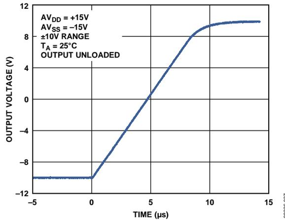
Figure 25. Full-Scale Positive Step
