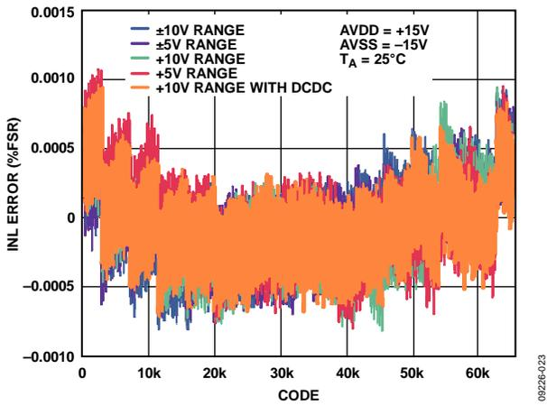
Figure 9. Integral Nonlinearity Error vs. DAC Code
