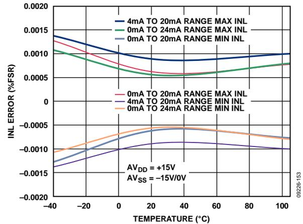
Figure 37. Integral Nonlinearity vs. Temperature, External RSET
