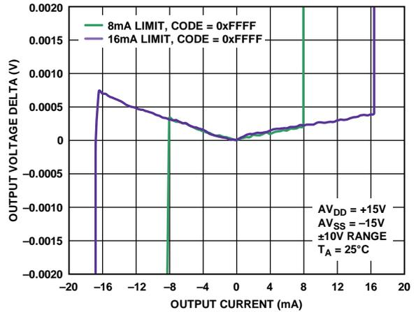
Figure 24. Source and Sink Capability of Output Amplifier
