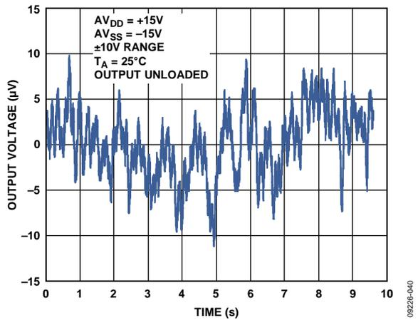
Figure 28. Peak-to-Peak Noise (0.1 Hz to 10 Hz Bandwidth)
