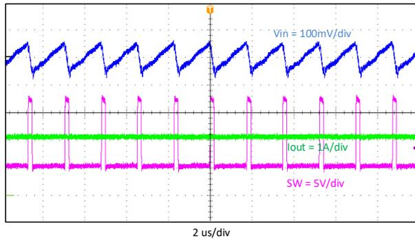
**Figure 9-4. Input Voltage Ripple  $I_{out} = 2\text{ A}$**
