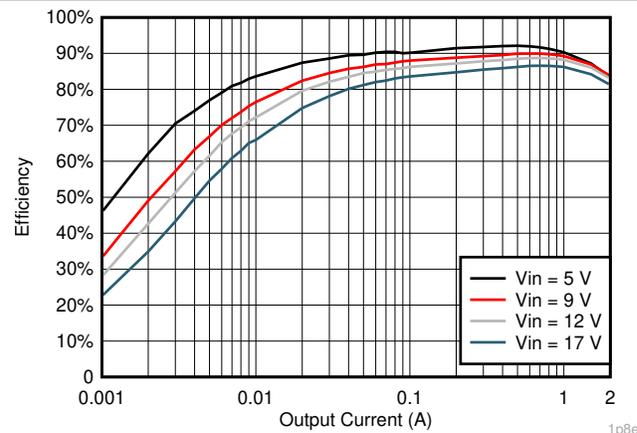
Figure 7-12.  $V_{OUT} = 1.8\text{-V}$  Efficiency,  $L = 2.2\ \mu\text{H}$
