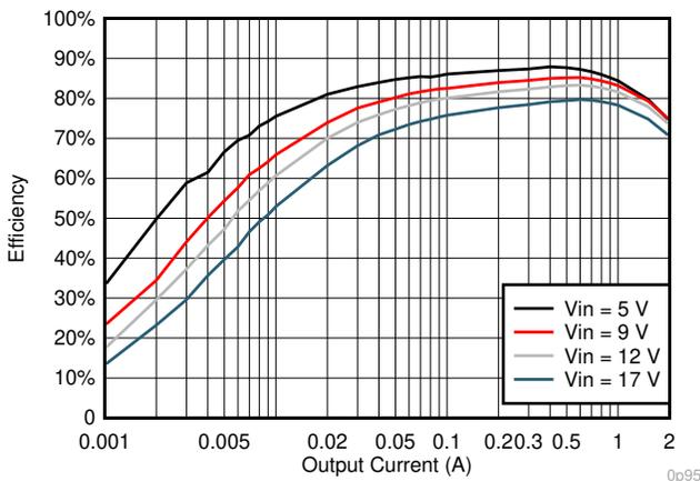
Figure 7-9.  $V_{OUT} = 0.95\text{-V}$  Efficiency,  $L = 2.2\ \mu\text{H}$
