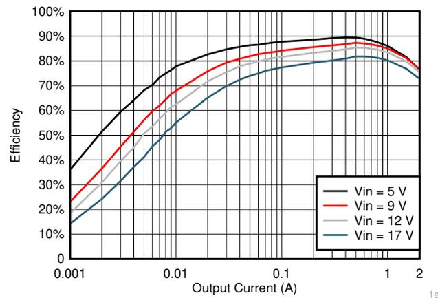
Figure 7-10.  $V_{OUT} = 1.05\text{-V}$  Efficiency,  $L = 2.2\ \mu\text{H}$
