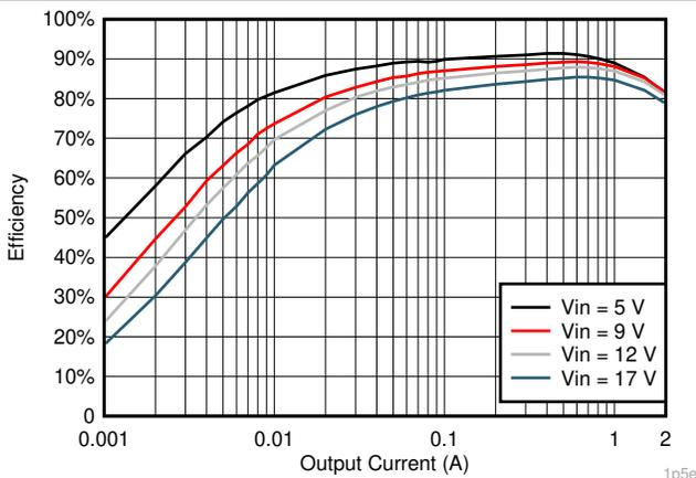
Figure 7-11.  $V_{OUT} = 1.5\text{-V}$  Efficiency,  $L = 2.2\ \mu\text{H}$
