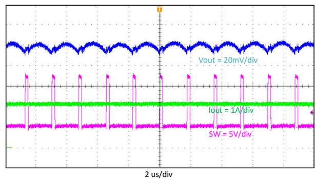
**Figure 9-7. Output Voltage Ripple,  $I_{out} = 2\text{ A}$**
