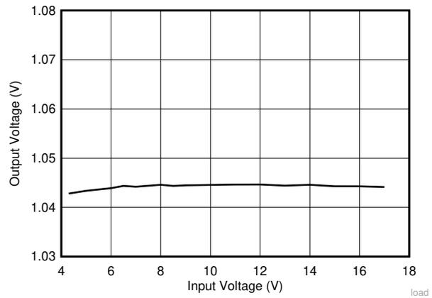
**Figure 9-3. Load Regulation with Different Input Voltage**
