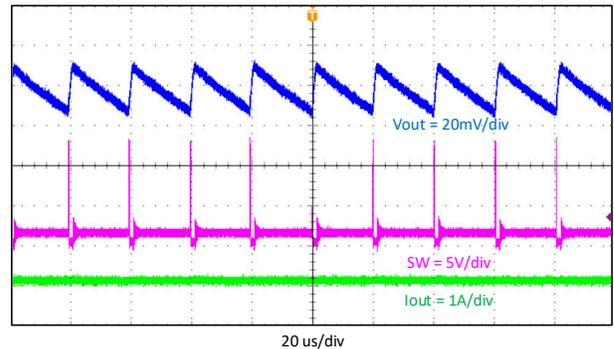
**Figure 9-5. Output Voltage Ripple,  $I_{out} = 0.01\text{ A}$**
