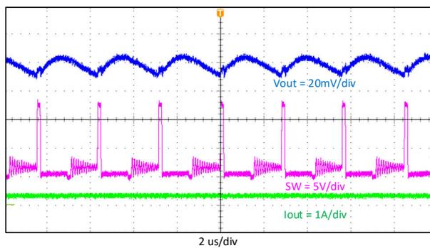
**Figure 9-6. Output Voltage Ripple,  $I_{out} = 0.2\text{ A}$**
