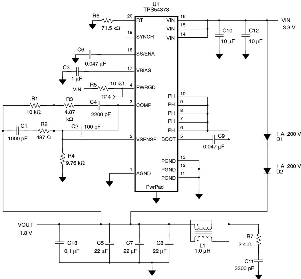
**Figure 10. Application Circuit**
