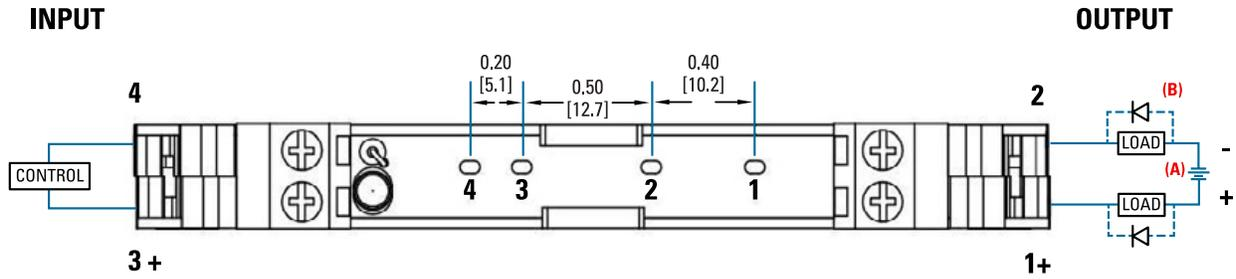
(A) Wiring diagram is identical for each individual section whether it is a single or four channel assembly.
