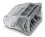
3-pos. socket terminal block with spring-cage connection, for toolless wiring with push-in connection method, for one and multi-strand conductors with a cross section of 0.5 to 2.5 mm², insulation housing transparent.
