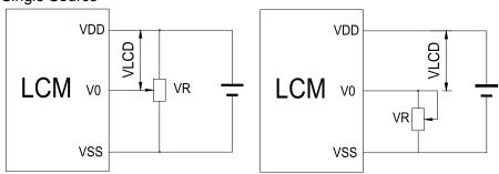
V<sub>DD∼</sub>V₀: LCD Driving voltage
