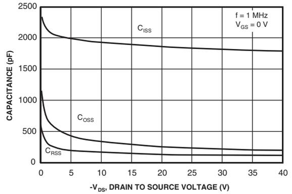
**Figure 8. Capacitance Characteristics.**
