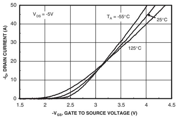
**Figure 5. Transfer Characteristics.**
