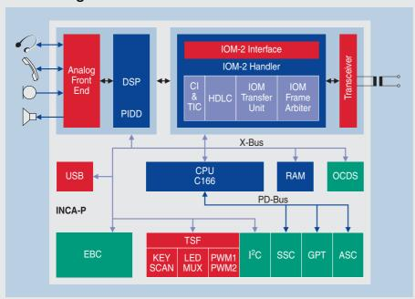
The typical application of the INCA-P is for terminal equipment in which the microphone, loud-speaker, headset, and handset are directly connected to the Analog Front End.
