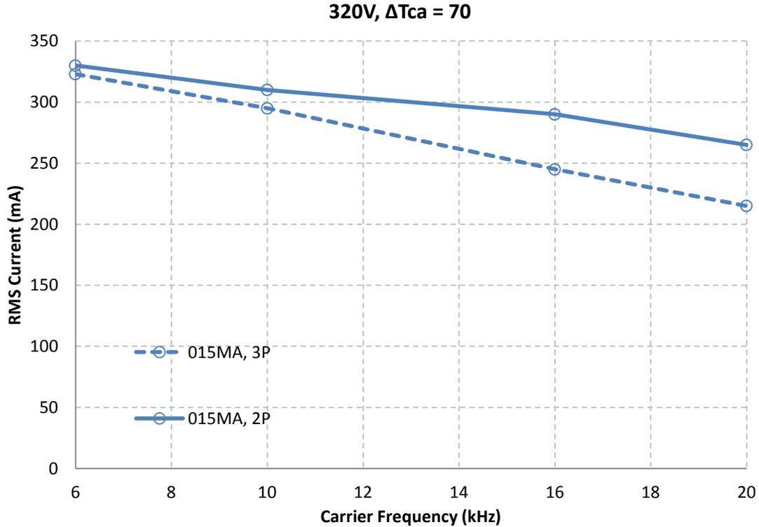
**Figure 6:** Maximum Sinusoidal Phase Current vs. PWM Switching Frequency
