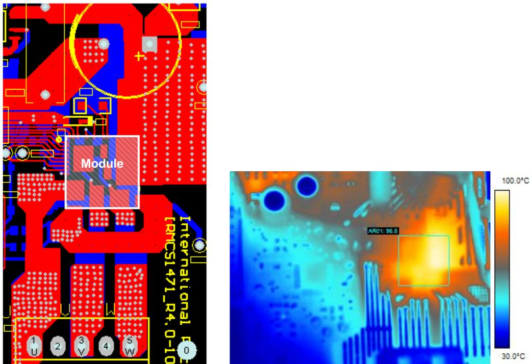
**Figure 7:** PCB layout example and corresponding thermal image (10kHz, 3P, 1oz,  $\Delta T_{ca}=70^{\circ}\text{C}$ ,  $V_+ = 320\text{V}$ ,  $I_u = 295\text{mA}$ )
