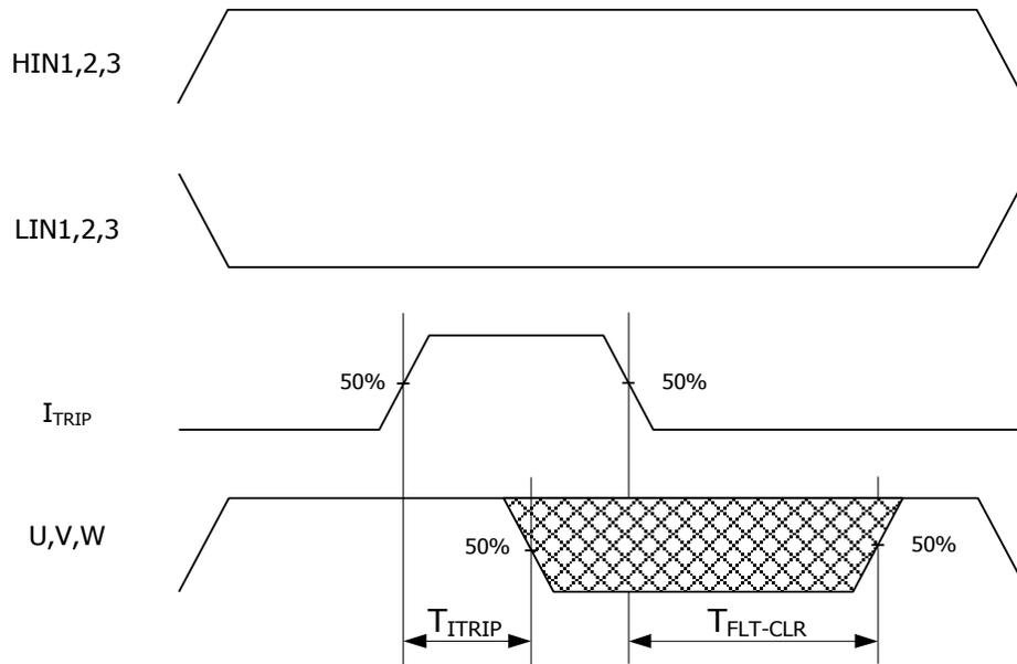
**Figure 3: I<sub>TRIP</sub> Timing Waveform**
