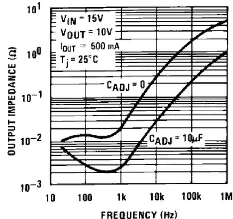
**Figure 12. Output Impedance**
