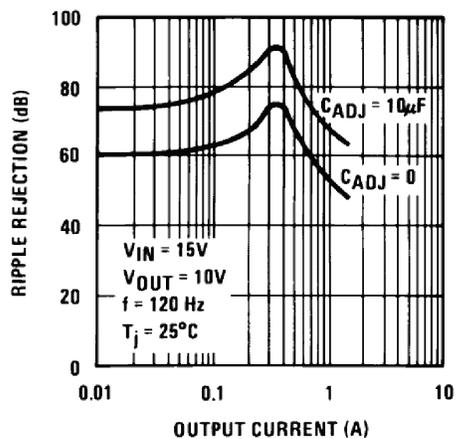
**Figure 11. Ripple Rejection**
