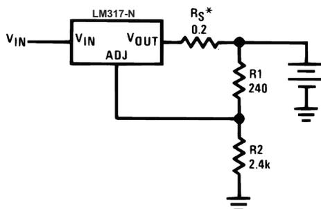
$$*R_S\text{—sets output impedance of charger: } Z_{OUT} = R_S \left( 1 + \frac{R_2}{R_1} \right)$$
