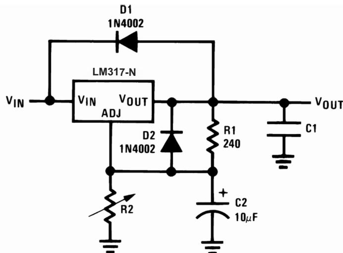
$$V_{OUT} = 1.25 V \left( 1 + \frac{R_2}{R_1} \right) + I_{ADJ} (R_2)$$
