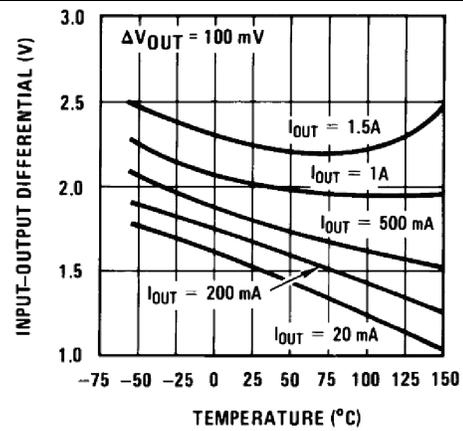
Figure 4. Dropout Voltage
