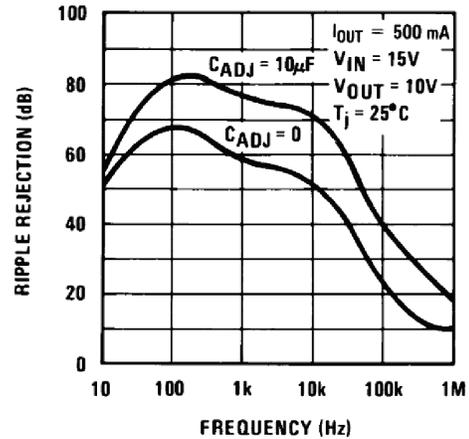
**Figure 10. Ripple Rejection**
