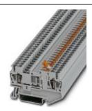
Knife disconnect terminal block, Connection type: Spring-cage connection, Cross section: 0.08 mm² - 4 mm², AWG: 28 - 12, Nominal current: 20 A, Nominal voltage: 400 V, Length: 60.5 mm, Width: 5.2 mm, Color: orange, Assembly: NS 35/7,5, NS 35/15
