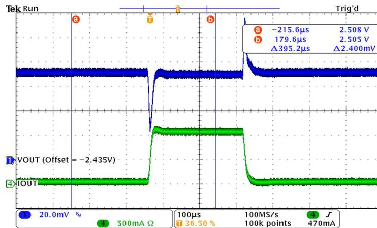
Figure 33. 1-A Load Transient Response ( $C_{OUT} = 10 \mu F$ )
