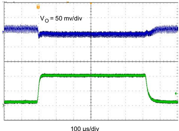
**Figure 8-11. TPS562201 Transient Response, 0.1 to 1.5 A**
