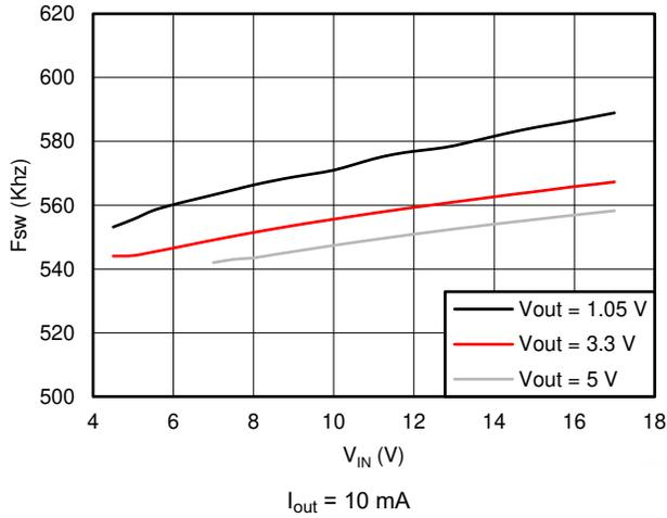
Figure 6-7. TPS562208 Switching Frequency vs Input Voltage
