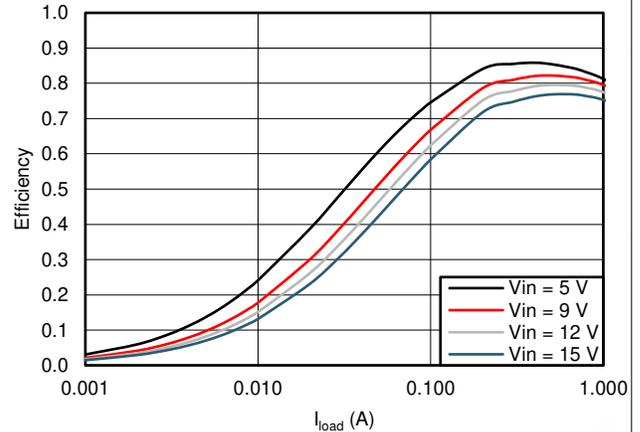
**Figure 6-14. TPS562208  $V_{OUT} = 1.05\text{ V}$  Efficiency,  $L = 2.2\ \mu\text{H}$**
