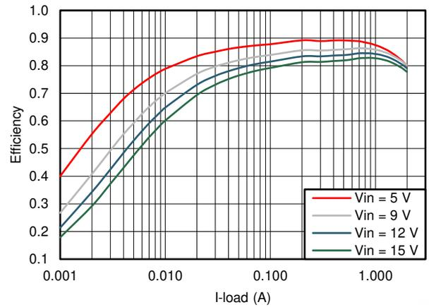
Figure 6-10. TPS562201  $V_{OUT} = 1.5\text{ V}$  Efficiency,  $L = 2.2\ \mu\text{H}$
