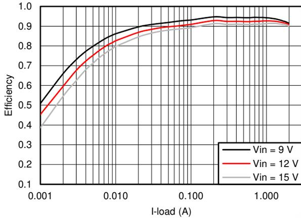
**Figure 6-13. TPS562201  $V_{OUT} = 5\text{ V}$  Efficiency,  $L = 3.3\ \mu\text{H}$**
