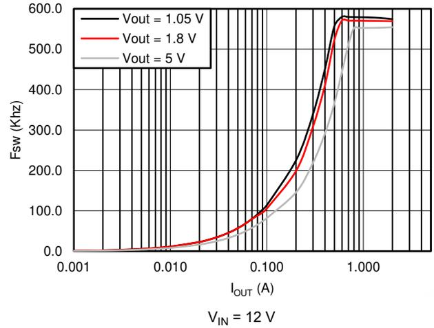
Figure 6-8. TPS562201 Switching Frequency vs Output Current
