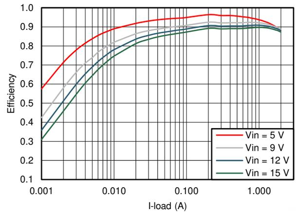
Figure 6-12. TPS562201  $V_{OUT} = 3.3\text{ V}$  Efficiency,  $L = 3.3\ \mu\text{H}$
