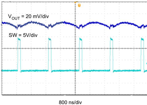
**Figure 8-10. TPS562208 Output Voltage Ripple,  $I_{OUT} = 0\text{ A}$**
