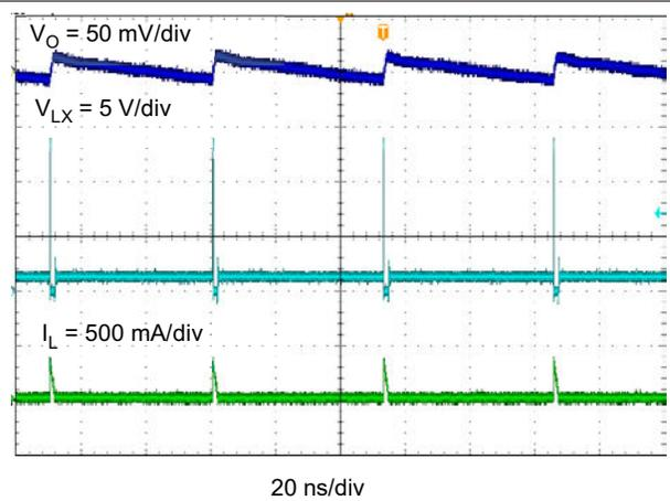
**Figure 8-7. TPS562201 Output Voltage Ripple,  $I_{OUT} = 10\text{ mA}$**
