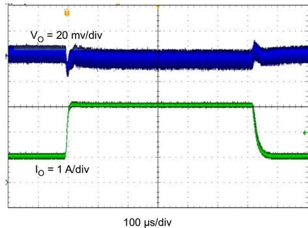
**Figure 8-12. TPS562201 Transient Response, 0.75 to 2.25 A**
