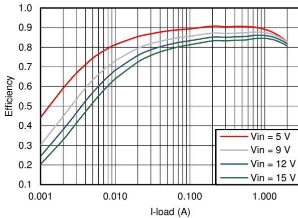
Figure 6-11. TPS562201  $V_{OUT} = 1.8\text{ V}$  Efficiency,  $L = 2.2\ \mu\text{H}$
