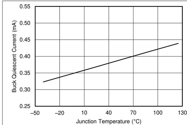
**Figure 6-1. TPS562201 Supply Current vs Junction Temperature**
