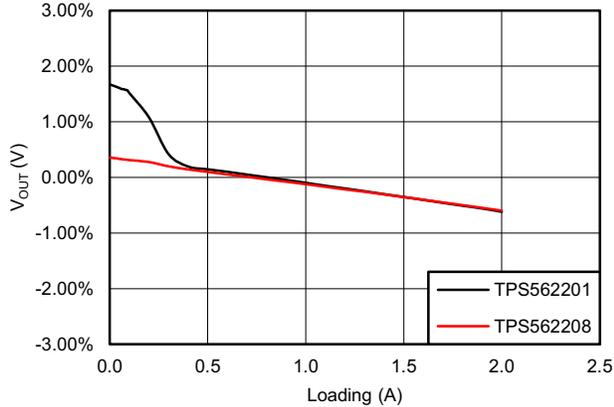
**Figure 8-2. Load Regulation,  $V_{IN} = 5\text{ V}$**
