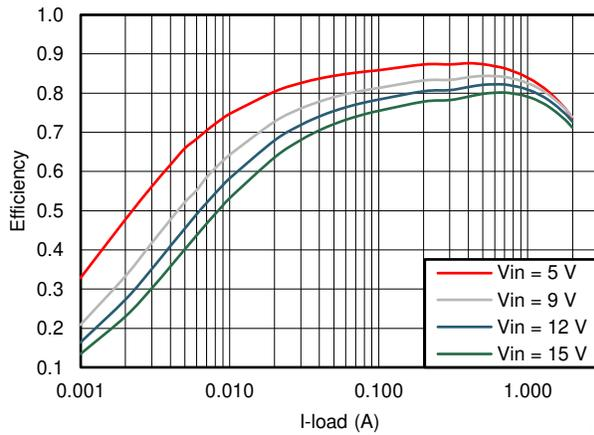
Figure 6-9. TPS562201  $V_{OUT} = 1.05\text{ V}$  Efficiency,  $L = 2.2\ \mu\text{H}$
