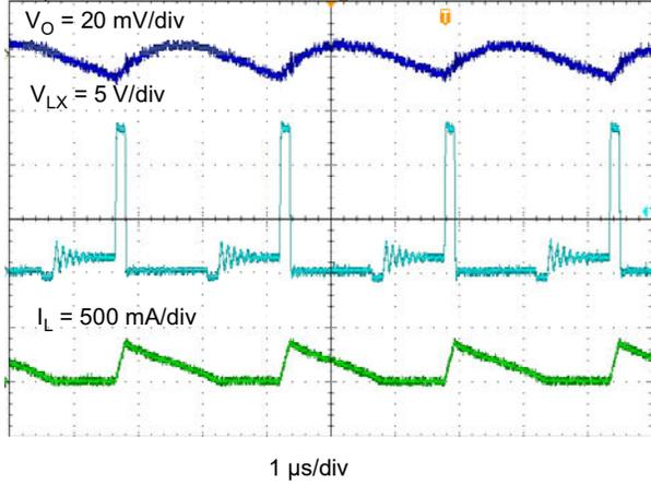
**Figure 8-8. TPS562201 Output Voltage Ripple,  $I_{OUT} = 0.25\text{ A}$**
