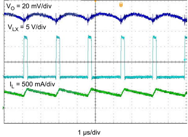
**Figure 8-9. TPS562201 Output Voltage Ripple,  $I_{OUT} = 2\text{ A}$**
