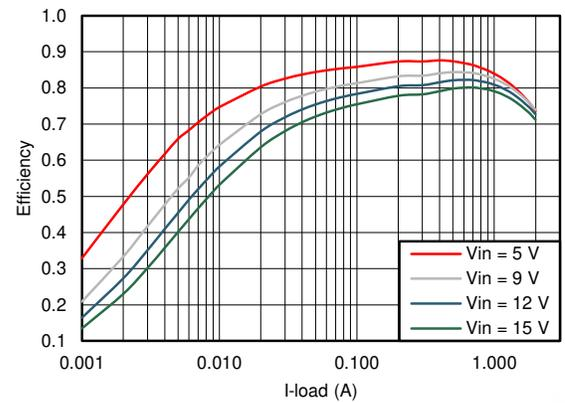
**Figure 8-5. TPS562201 Efficiency,  $V_{OUT} = 1.05\text{ V}$**
