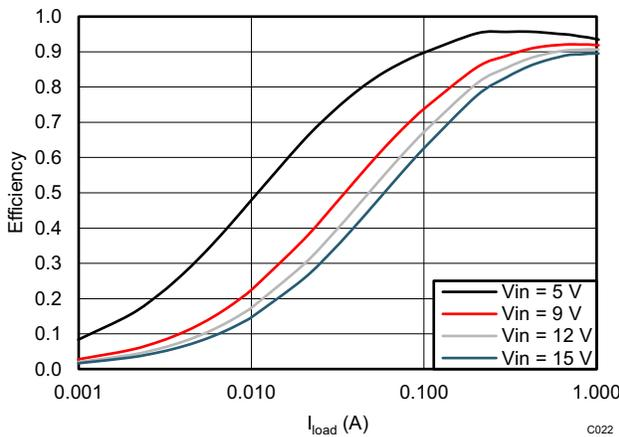
**Figure 6-17. TPS562208  $V_{OUT} = 3.3\text{ V}$  Efficiency,  $L = 2.2\ \mu\text{H}$**
