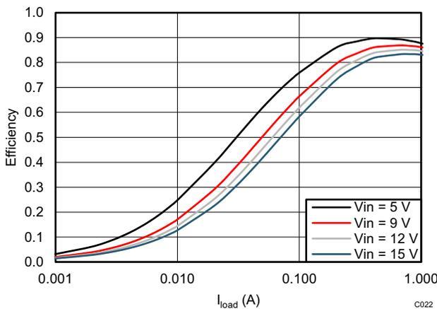
**Figure 6-15. TPS562208  $V_{OUT} = 1.5\text{ V}$  Efficiency,  $L = 2.2\ \mu\text{H}$**
