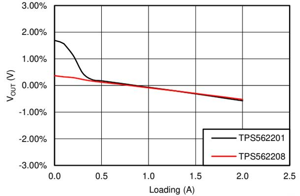
**Figure 8-3. Load Regulation  $V_{IN} = 12\text{ V}$**
