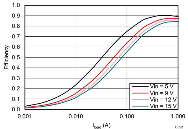
**Figure 6-16. TPS562208  $V_{OUT} = 1.8\text{ V}$  Efficiency,  $L = 2.2\ \mu\text{H}$**
