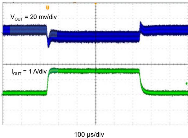
**Figure 8-13. TPS562208 Transient Response 0.1 to 2 A**
