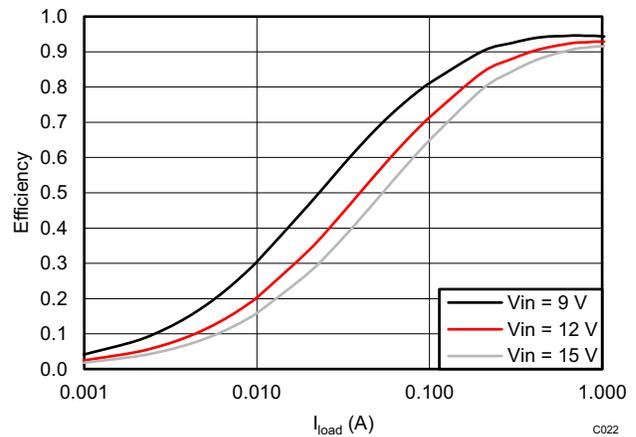
**Figure 6-18. TPS562208  $V_{OUT} = 5\text{ V}$  Efficiency,  $L = 3.3\ \mu\text{H}$**
