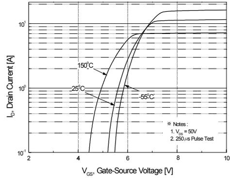
**Figure 2. Transfer Characteristics**
