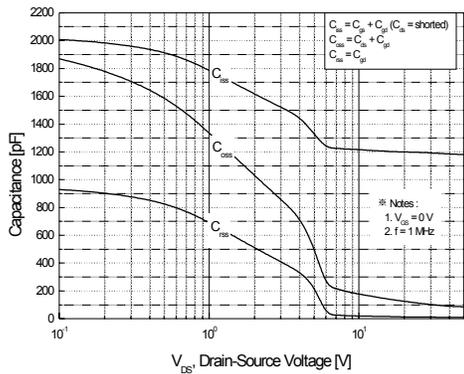
**Figure 5. Capacitance Characteristics**
