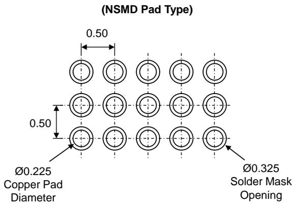
\* Dimensions are in millimeters.
