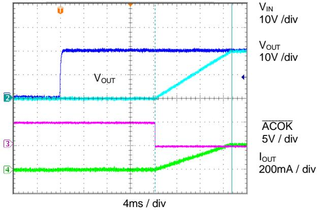
**OVP Response Time ( $V_{IN} = 20V$  to  $90V$  Surge)**
