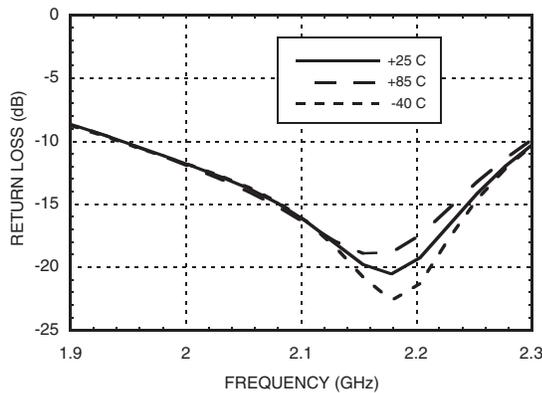
**Output Return Loss vs. Temperature @ 2100 MHz**
