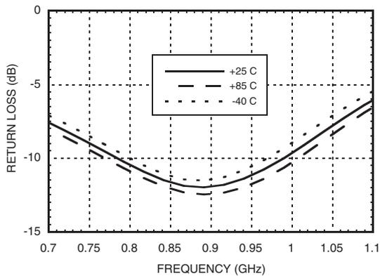
**Output Return Loss vs. Temperature @ 900 MHz**
