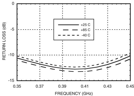
**Output Return Loss vs. Temperature @ 400 MHz**
