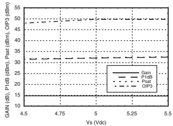
**Gain, Power & IP3 vs. Supply Current @ 900 MHz\***
