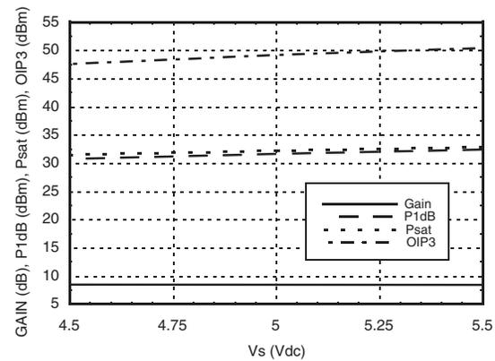
**Gain, Power & IP3 vs. Supply Current @ 1900 MHz\***
