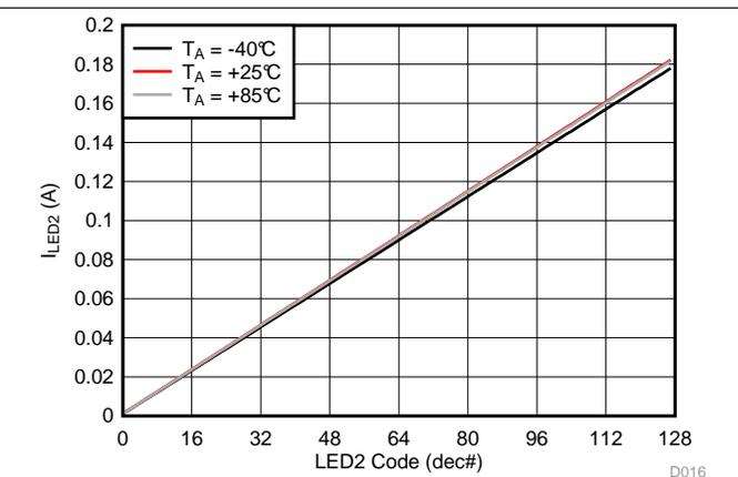
Figure 5. LED2 Torch Current vs Brightness Code
