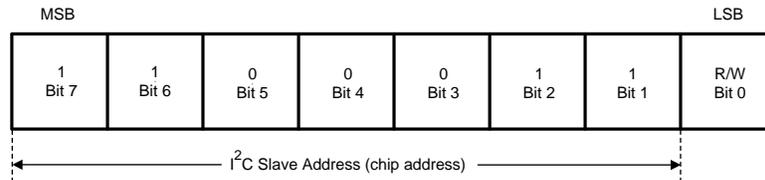
Figure 35. I<sup>2</sup>C-Compatible Chip Address
