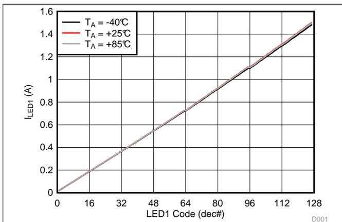
Figure 2. LED1 Flash Current vs Brightness Code
