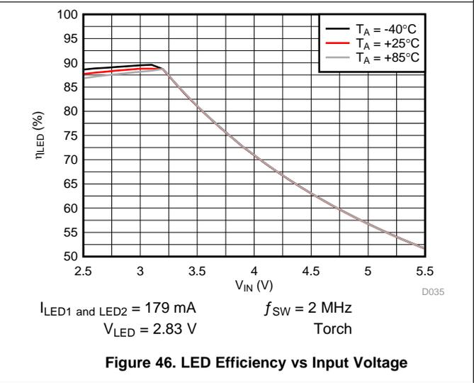
Ambient temperature is 25°C, input voltage is 3.6V, HWEN = V<sub>IN</sub>, C<sub>IN</sub> = 2 × 10 μF, C<sub>OUT</sub> = 2 × 10 μF and L = 1 μH, unless otherwise noted.
