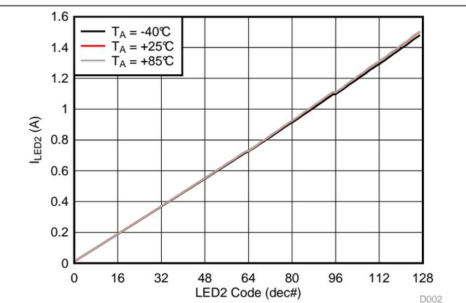
Figure 3. LED2 Flash Current vs Brightness Code
