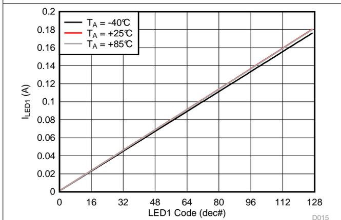
Figure 4. LED1 Torch Current vs Brightness Code
