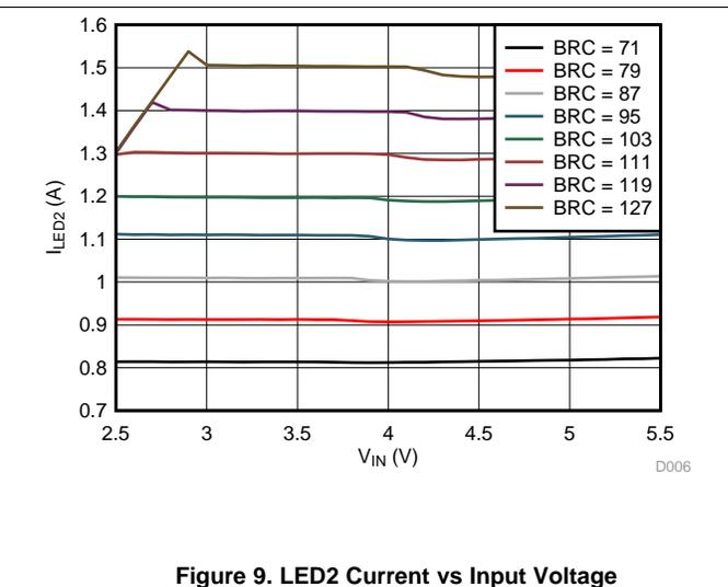
Figure 9. LED2 Current vs Input Voltage
