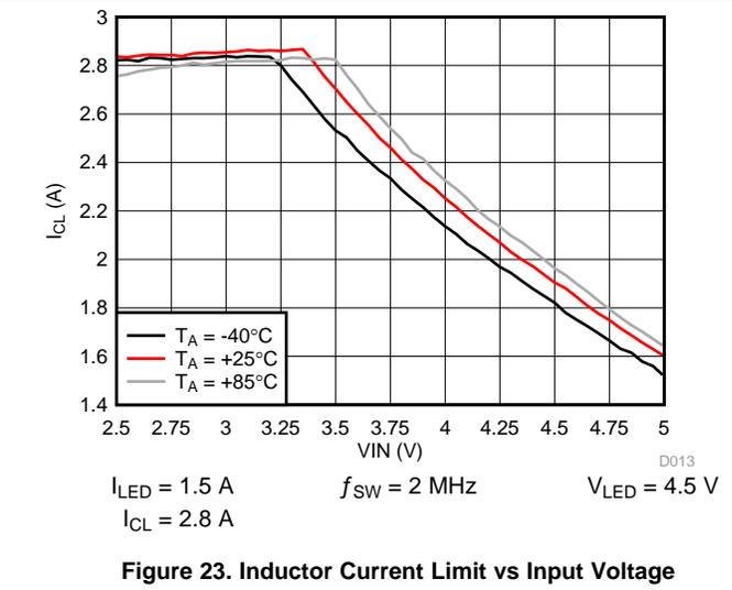
Figure 23. Inductor Current Limit vs Input Voltage
