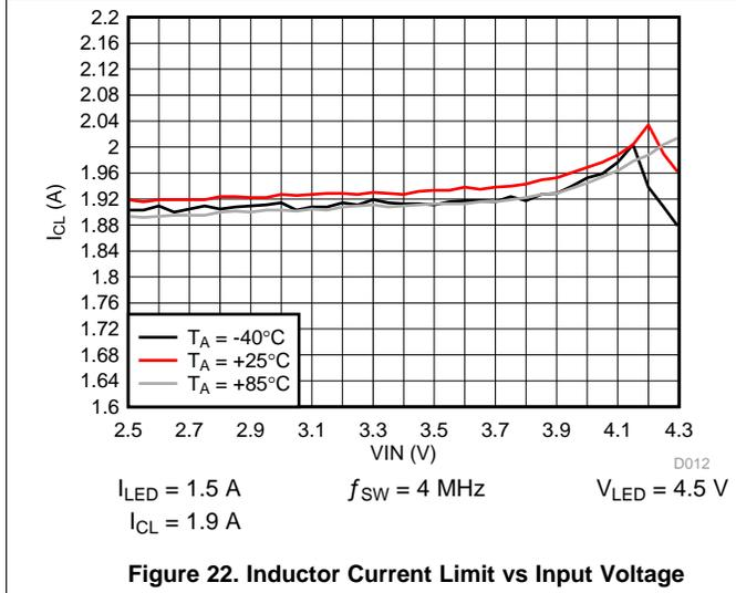
Figure 22. Inductor Current Limit vs Input Voltage
