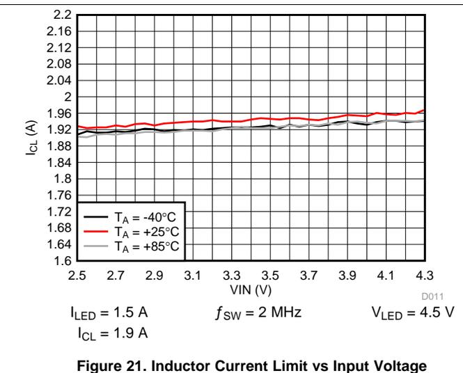
Figure 21. Inductor Current Limit vs Input Voltage
