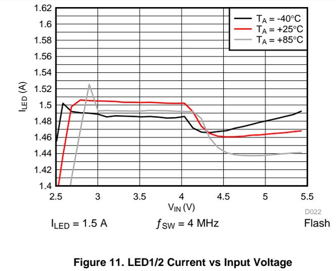
Figure 11. LED1/2 Current vs Input Voltage
