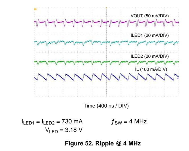
Ambient temperature is 25°C, input voltage is 3.6V, HWEN = V<sub>IN</sub>, C<sub>IN</sub> = 2 × 10 μF, C<sub>OUT</sub> = 2 × 10 μF and L = 1 μH, unless otherwise noted.
