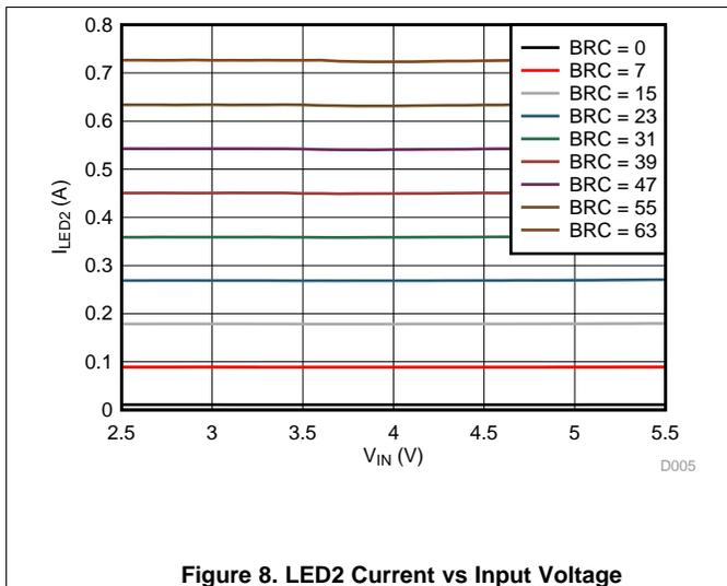
Figure 8. LED2 Current vs Input Voltage
