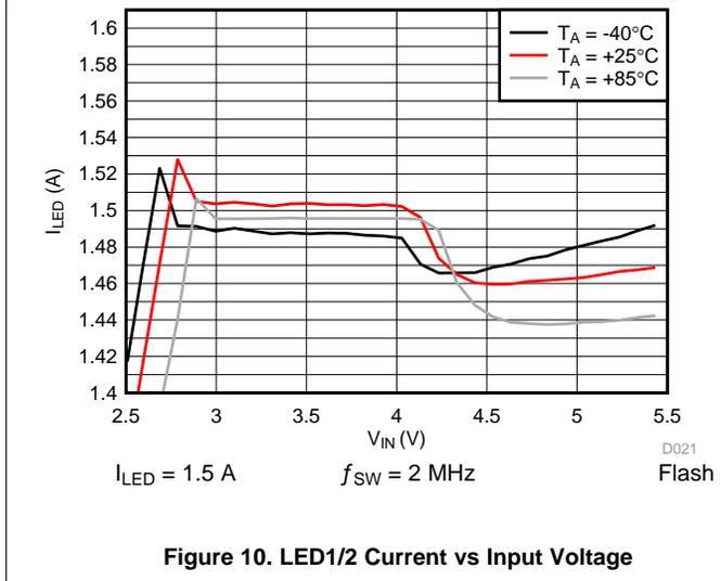
Figure 10. LED1/2 Current vs Input Voltage
