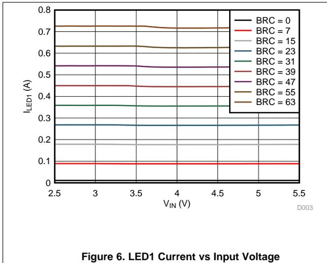
Figure 6. LED1 Current vs Input Voltage
