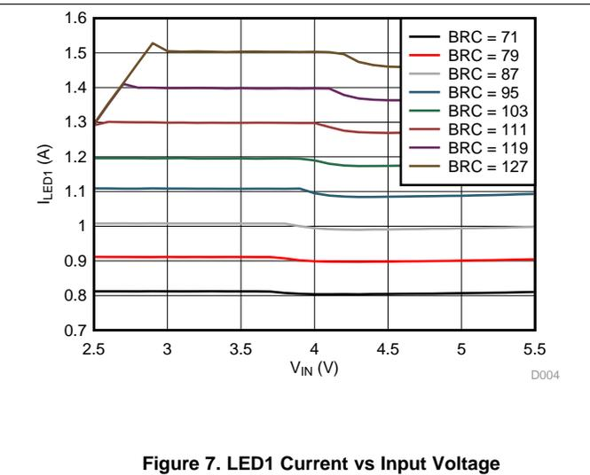
Figure 7. LED1 Current vs Input Voltage
