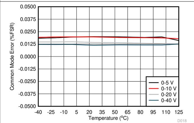
**Figure 7-20. Common Mode Error vs Temperature (Differential Unipolar Outputs)**
