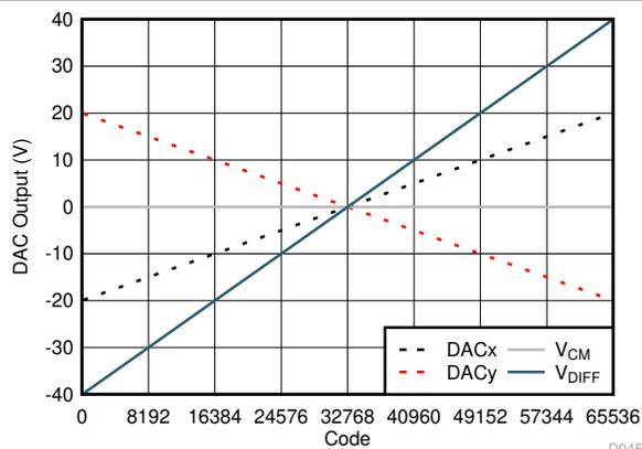
**Figure 8-2. Differential Bipolar Output (16-Bit):
