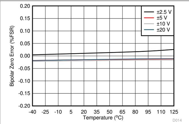
**Figure 7-16. Bipolar Zero Error vs Temperature**
