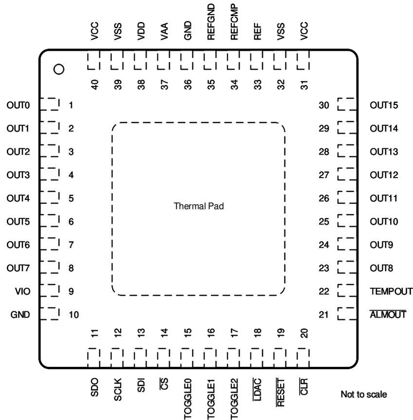
Figure 6-1. RHA Package, 40-Pin VQFN, Top View
