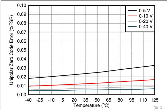
**Figure 7-15. Unipolar Zero Code Error vs Temperature**
