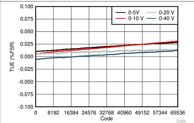
**Figure 7-8. Total Unadjusted Error vs Digital Input Code (Unipolar Outputs)**
