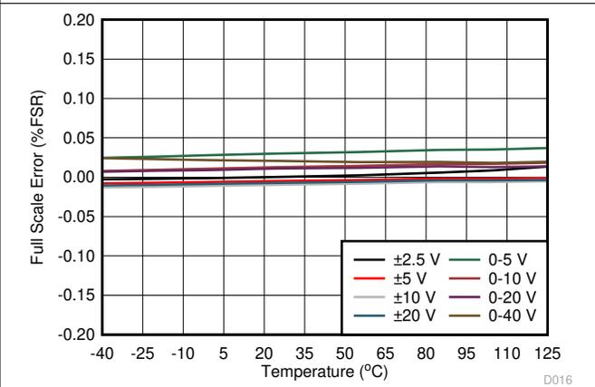
**Figure 7-18. Full-Scale Error vs Temperature**
