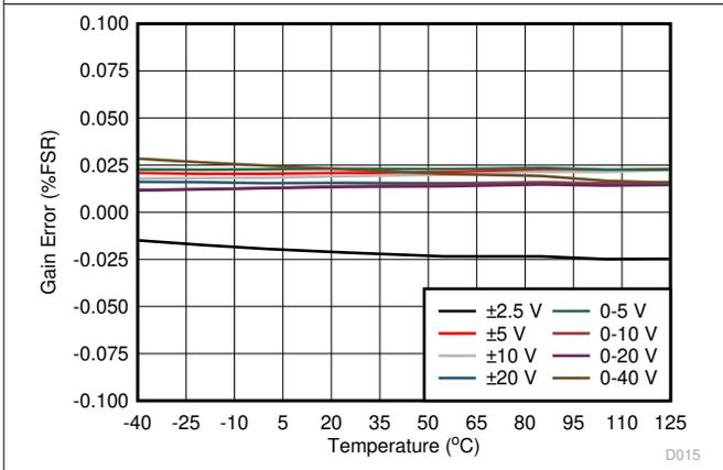
**Figure 7-17. Gain Error vs Temperature**
