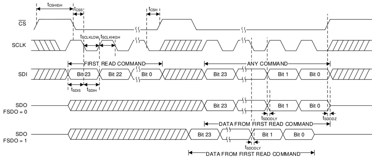
**Figure 7-2. Serial Interface Read Timing Diagram**
