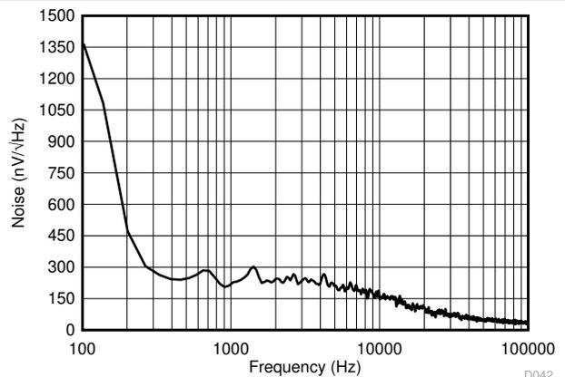
**Figure 7-44. Internal Reference Noise Density vs Frequency**
