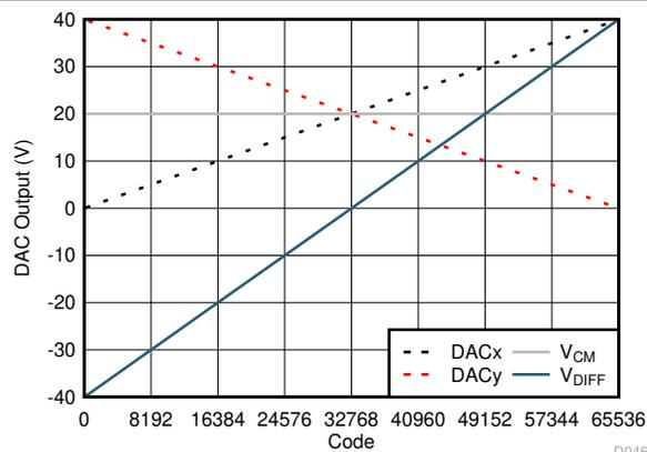
**Figure 8-3. Differential Unipolar Output (16-Bit):
