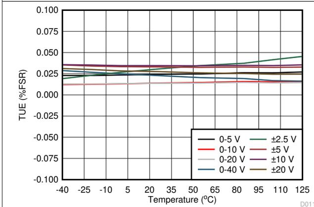
**Figure 7-13. Total Unadjusted Error vs Temperature**
