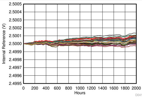
**Figure 7-43. Internal Reference Voltage vs Time**
