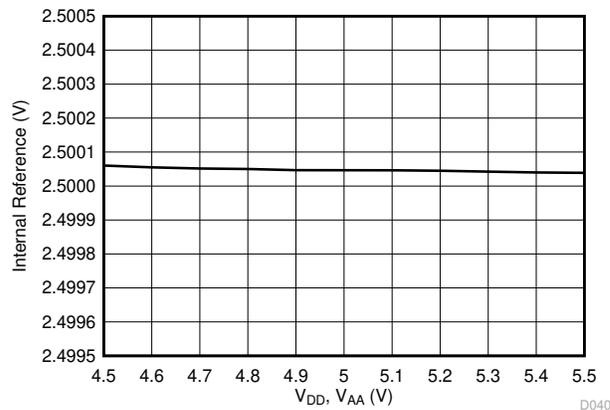
**Figure 7-42. Internal Reference Voltage vs Supply Voltage**
