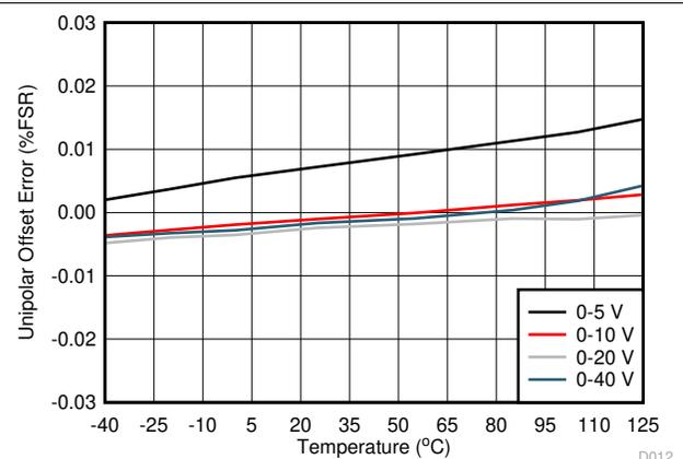
**Figure 7-14. Unipolar Offset Error vs Temperature**
