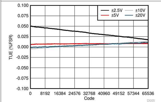
**Figure 7-7. Total Unadjusted Error vs Digital Input Code (Bipolar Outputs)**
