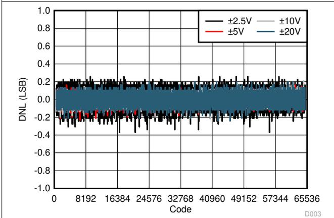
**Figure 7-5. Differential Linearity Error vs Digital Input Code (Bipolar Outputs)**
