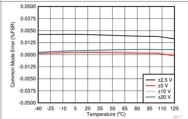
**Figure 7-19. Common Mode Error vs Temperature (Differential Bipolar Outputs)**
