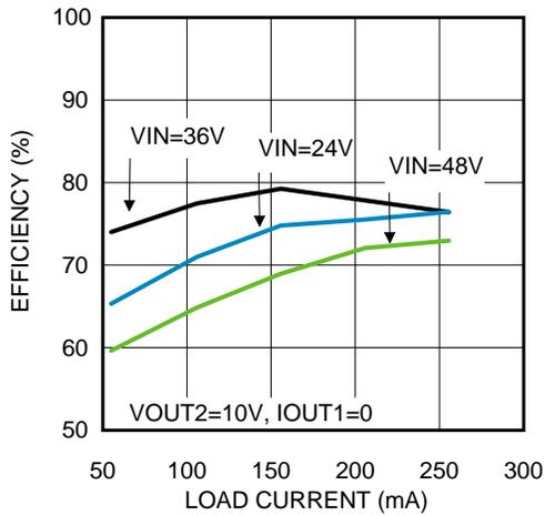
Figure 1. Efficiency at 750 kHz,  $V_{OUT1} = 10\text{ V}$
