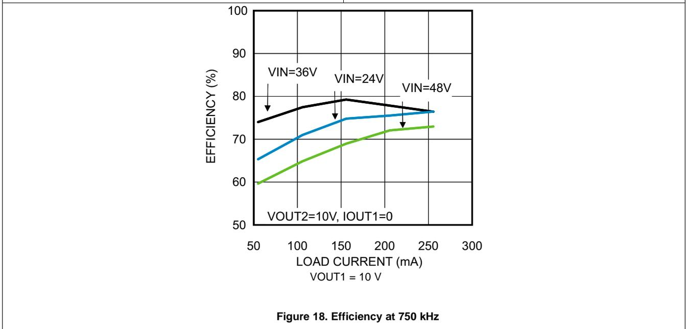
Figure 18. Efficiency at 750 kHz
