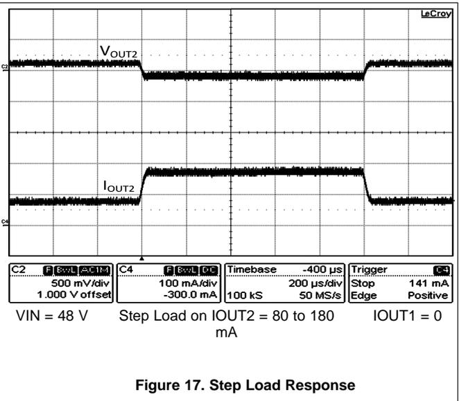
Figure 17. Step Load Response
