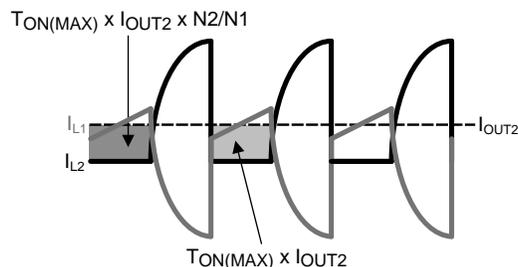
Figure 13. Current Waveforms for  $C_{\text{OUT1}}$  Ripple Calculation
