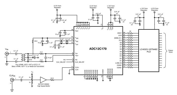
Figure 23. Application Circuit using Transformer Drive Circuit (If 14-bit compatibility is not required do not connect pins 17 and 18)
