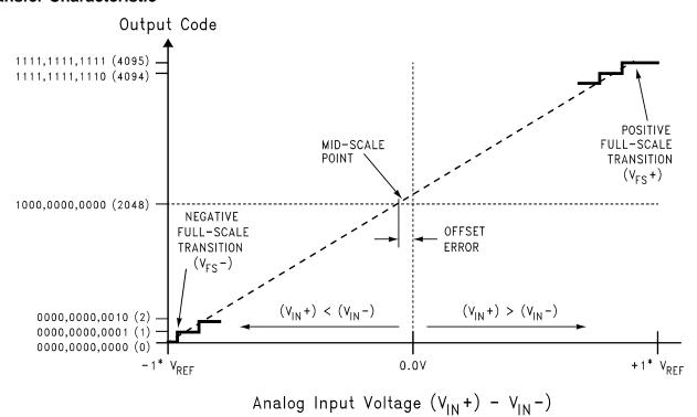
Figure 2. Transfer Characteristic (Offset Binary Format)
