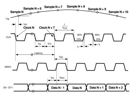
Figure 1. Output Timing
