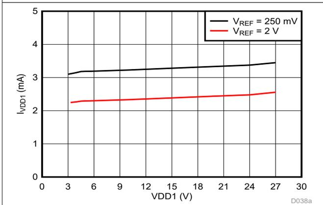
Figure 6-43. High-Side Supply Current vs Supply Voltage
