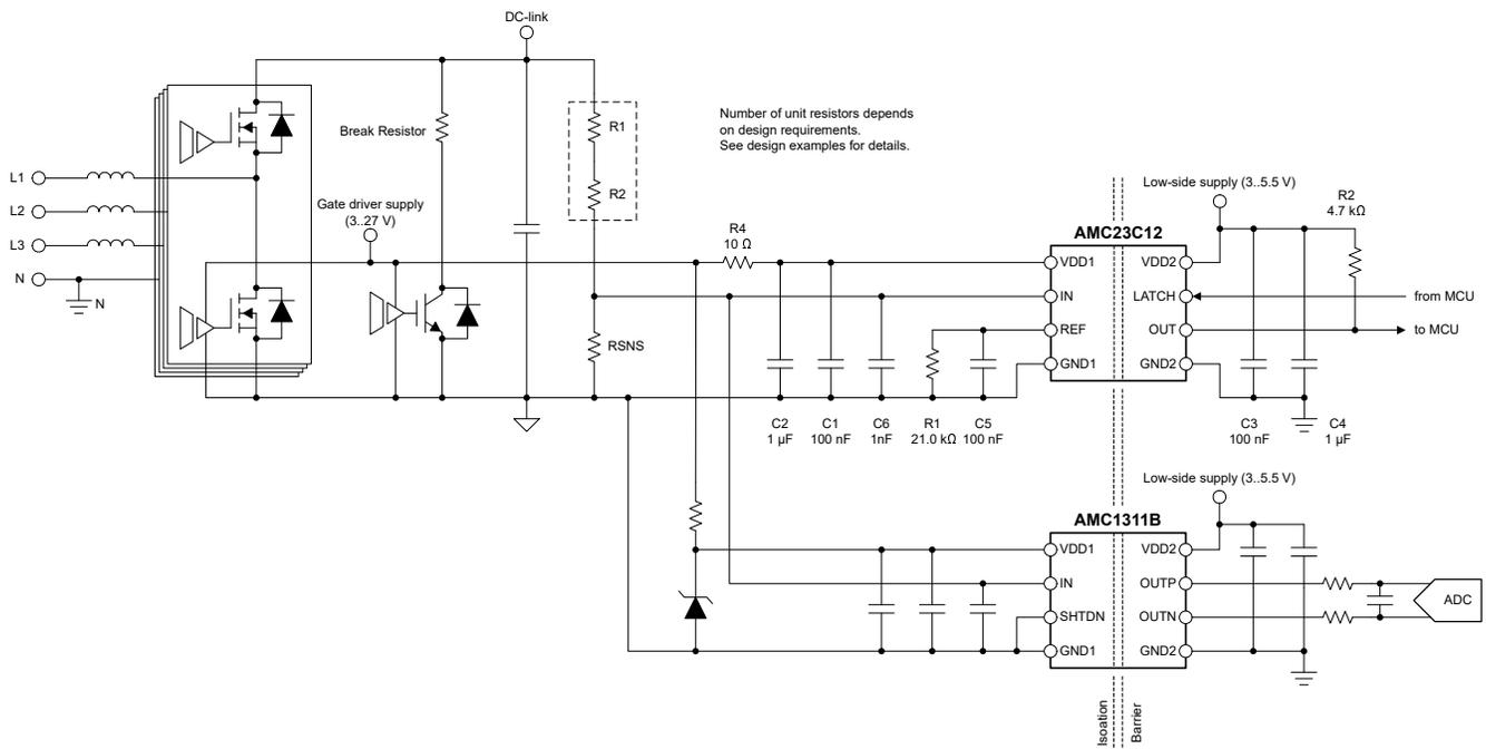
Figure 8-2. Using the AMC23C12 for Overvoltage Detection
