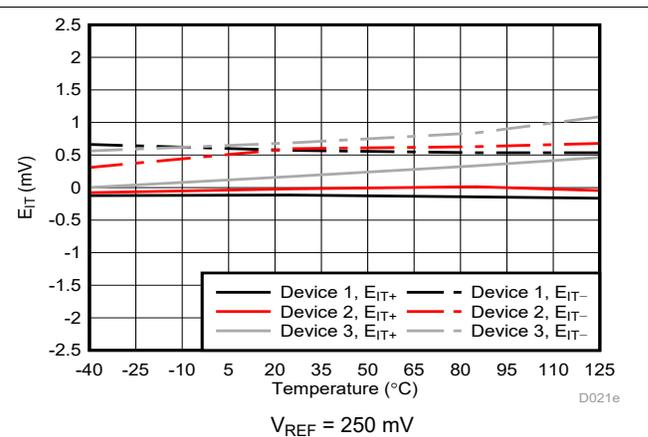
Figure 6-14. Cmp0 Trip Threshold Error vs Temperature
