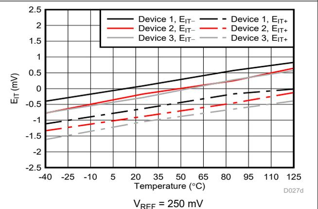
Figure 6-32. Cmp1 Trip Threshold Error vs Temperature
