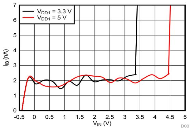
Figure 6-39. Input Bias Current vs Input Voltage
