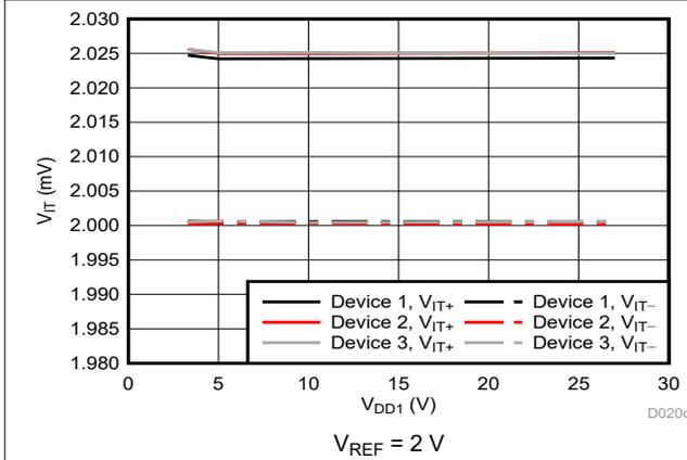
Figure 6-17. Cmp0 Trip Threshold vs Supply Voltage
