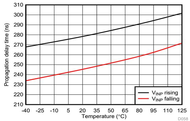
Figure 6-38. Cmp1 Propagation Delay vs Temperature
