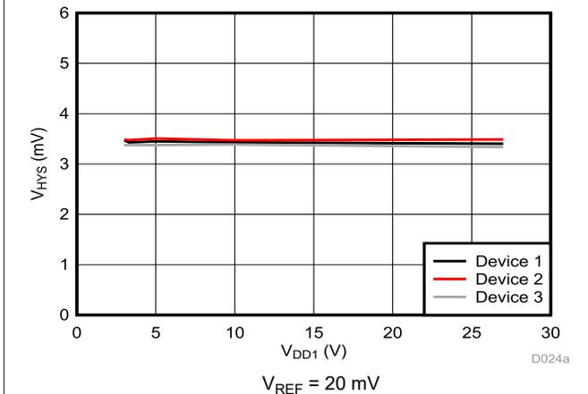
Figure 6-9. Cmp0 Trip Threshold Hysteresis vs Supply Voltage
