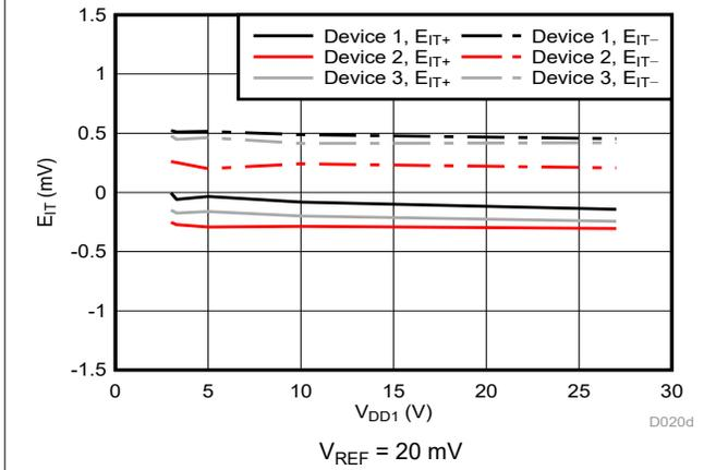
Figure 6-7. Cmp0 Trip Threshold Error vs Supply Voltage
