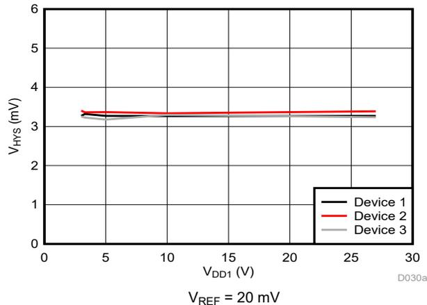
Figure 6-27. Cmp1 Trip Threshold Hysteresis vs Supply Voltage
