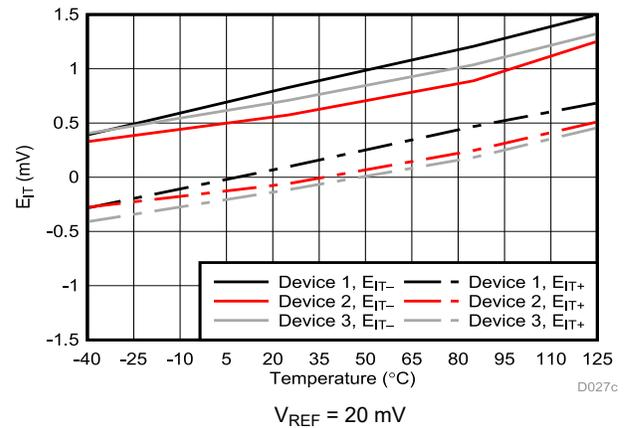
Figure 6-26. Cmp1 Trip Threshold Error vs Temperature
