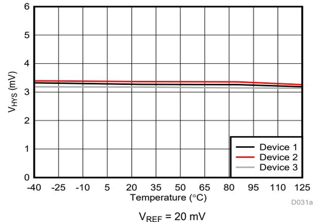
Figure 6-28. Cmp1 Trip Threshold Hysteresis vs Temperature
