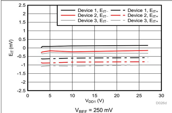
Figure 6-31. Cmp1 Trip Threshold Error vs Supply Voltage
