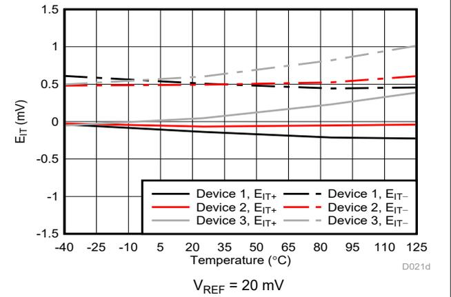
Figure 6-8. Cmp0 Trip Threshold Error vs Temperature
