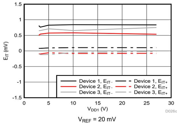
Figure 6-25. Cmp1 Trip Threshold Error vs Supply Voltage
