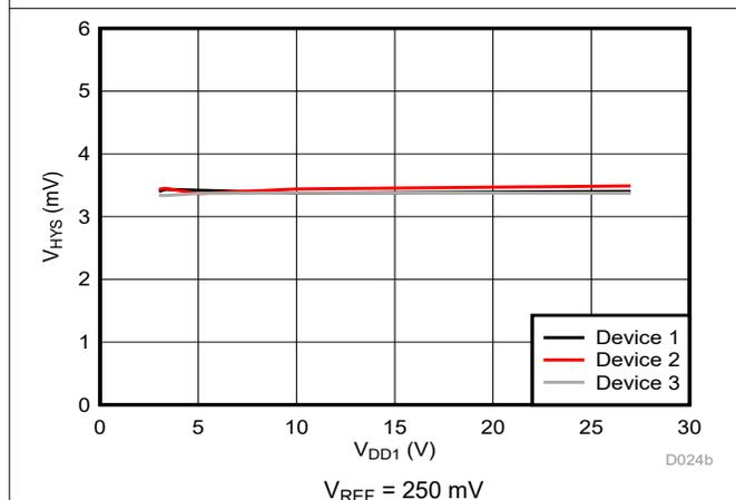
Figure 6-15. Cmp0 Trip Threshold Hysteresis vs Supply Voltage
