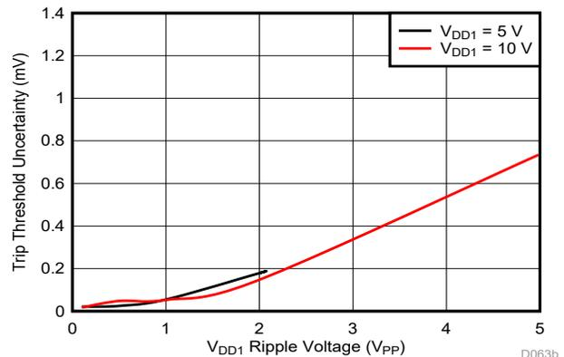
Figure 8-5. Trip Threshold Sensitivity to VDD1 Ripple Voltage (Cmp1, f<sub>RIPPLE</sub> = 10 kHz)
