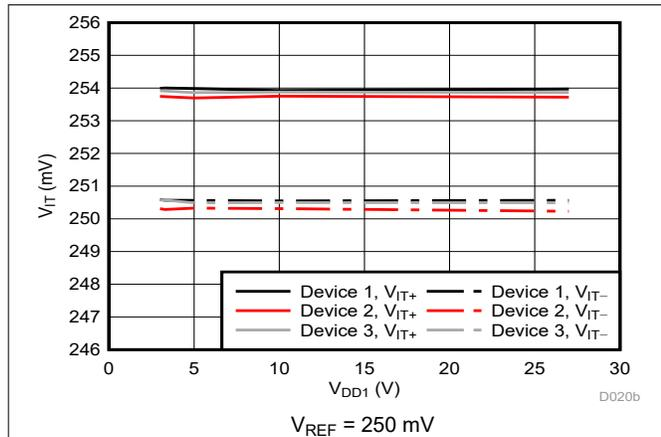
Figure 6-11. Cmp0 Trip Threshold vs Supply Voltage
