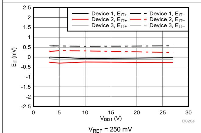
Figure 6-13. Cmp0 Trip Threshold Error vs Supply Voltage
