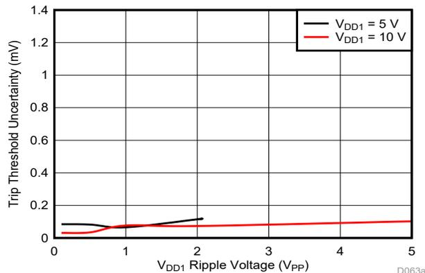
Figure 8-4. Trip Threshold Sensitivity to VDD1 Ripple Voltage (Cmp0, f<sub>RIPPLE</sub> = 10 kHz)
