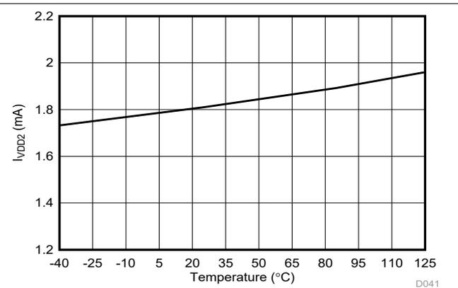
Figure 6-46. Low-Side Supply Current vs Temperature
