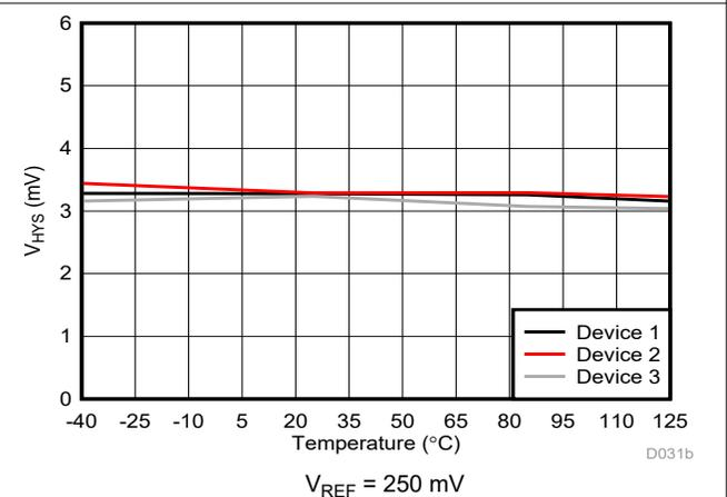
Figure 6-34. Cmp1 Trip Threshold Hysteresis vs Temperature
