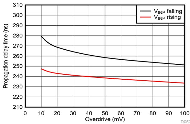
Figure 6-37. Cmp1 Propagation Delay vs Overdrive
