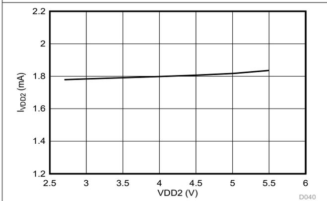
Figure 6-45. Low-Side Supply Current vs Supply Voltage
