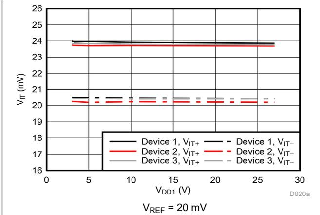
Figure 6-5. Cmp0 Trip Threshold vs Supply Voltage
