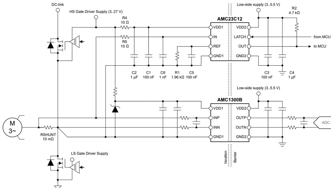
**Figure 8-1. Using the AMC23C12 for Overcurrent Detection**
