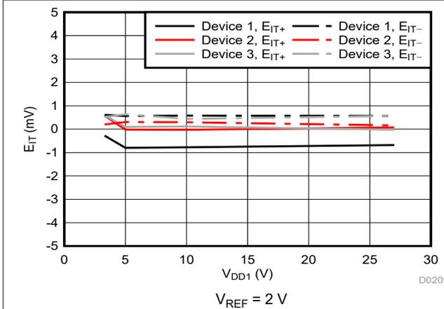
Figure 6-19. Cmp0 Trip Threshold Error vs Supply Voltage
