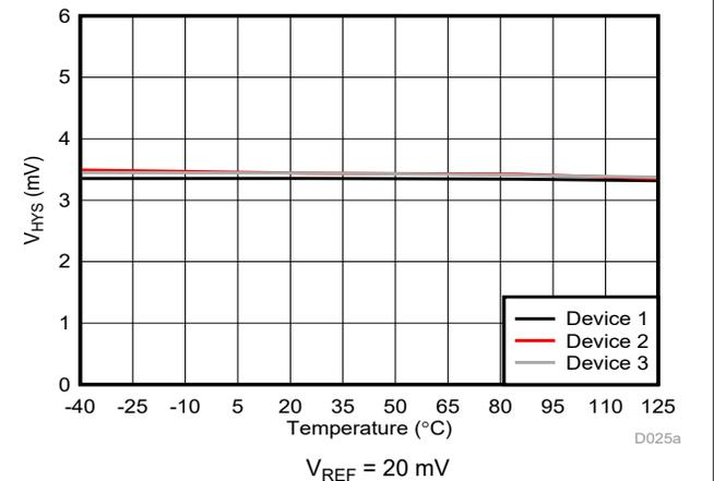
Figure 6-10. Cmp0 Trip Threshold Hysteresis vs Temperature
