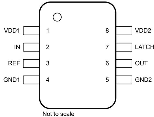
**Figure 5-1. DWV Package, 8-Pin SOIC (Top View)**
