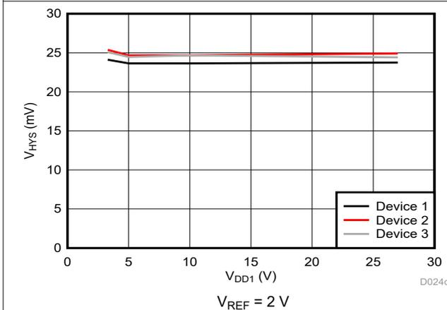
Figure 6-21. Cmp0 Trip Threshold Hysteresis vs Supply Voltage
