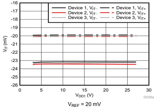
Figure 6-23. Cmp1 Trip Threshold vs Supply Voltage
