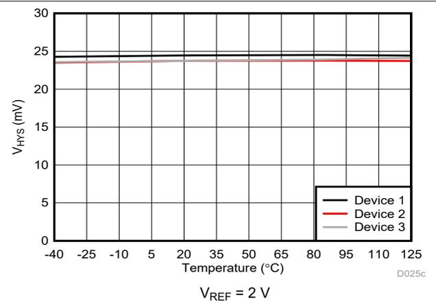
Figure 6-22. Cmp0 Trip Threshold Hysteresis vs Temperature
