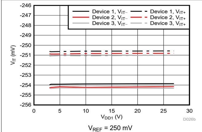
Figure 6-29. Cmp1 Trip Threshold vs Supply Voltage
