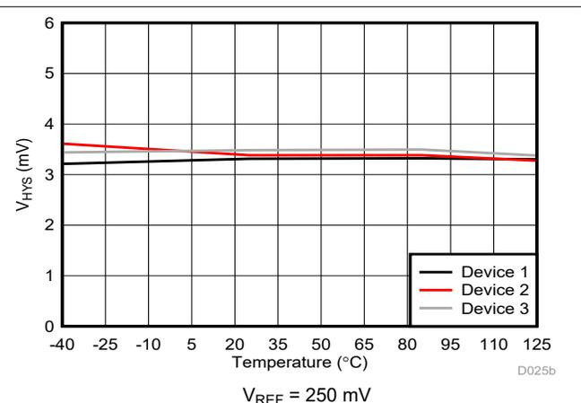
Figure 6-16. Cmp0 Trip Threshold Hysteresis vs Temperature
