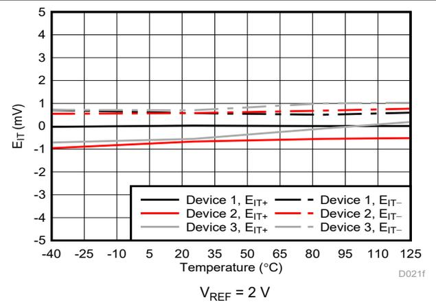
Figure 6-20. Cmp0 Trip Threshold Error vs Temperature
