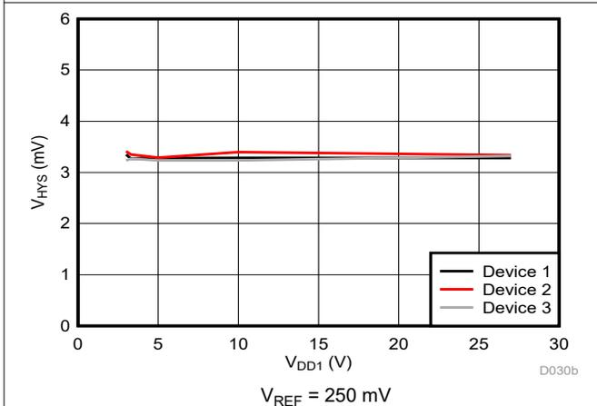
Figure 6-33. Cmp1 Trip Threshold Hysteresis vs Supply Voltage
