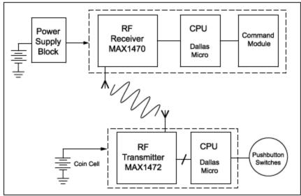
Figure 1. An RKE system consists of a keyfob circuit (lower diagram) transmitting to a receiver in the vehicle (upper diagram).
