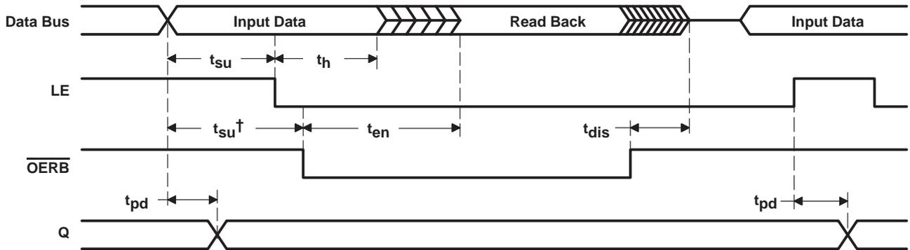
† This setup time ensures that the read-back circuit will not create a conflict on the input data bus.
