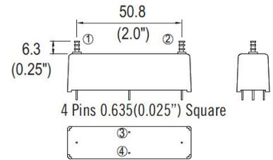
NOTE: PINS WHICH ARE NOT NUMBERED HAVE NO ELECTRICAL CONNECTION.
