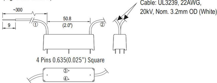
NOTE: PINS WHICH ARE NOT NUMBERED HAVE NO ELECTRICAL CONNECTION.
