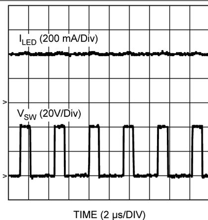
Figure 11. Steady-State Operation ( $I_{LED} = 0.2\text{ A}$ )
