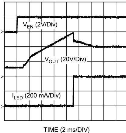
Figure 10. Enable Transient ( $I_{LED} = 0.2\text{ A}$ )
