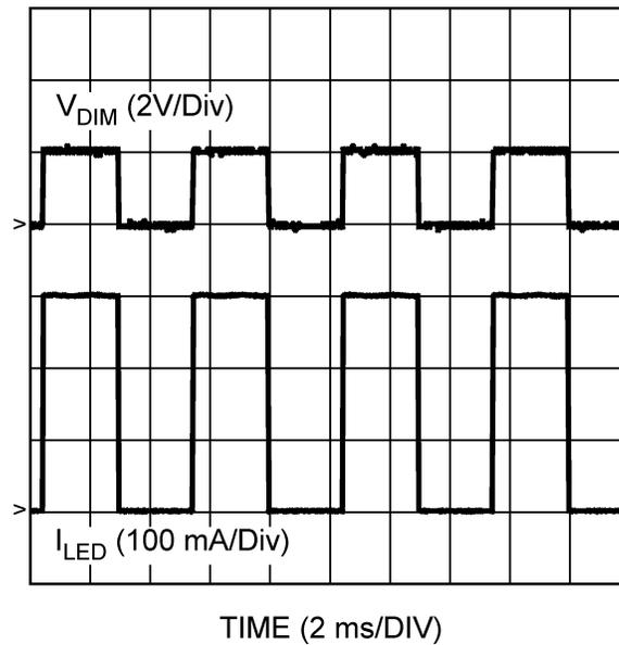
**Figure 27. LED 50% Dimming, Both Channels Combined**
