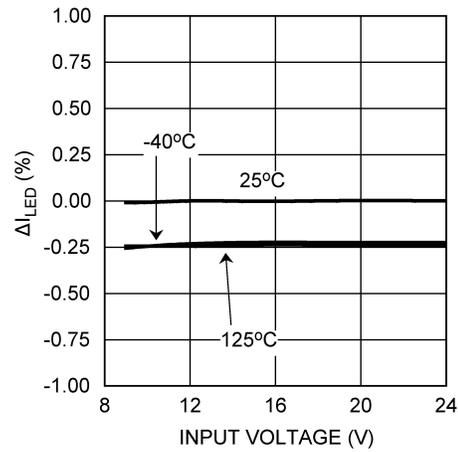
Figure 8.  $I_{LED}$  Regulation vs  $V_{IN}$  ( $I_{LED} = 0.2\text{ A}$ )
