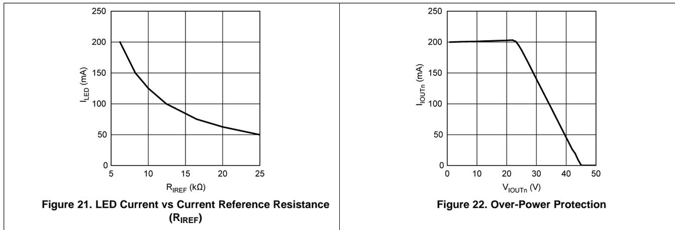
If the voltage on the IOU<sub>Tn</sub> (n = 1, 2) pin is higher than 24 V when channel n is on, the regulated current of channel n reduces linearly if the voltage further increases (as shown in Figure 22). The regulated current of another channel is not affected. This over-power protection feature avoids damaging the current regulator owing to the shorting of many LEDs in one string.
