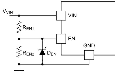
**Figure 19. Input Voltage UVLO Implemented by Precision Enable**
