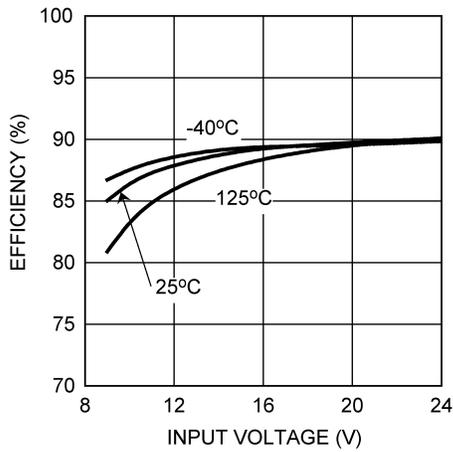
Figure 7. Efficiency vs  $V_{IN}$  ( $I_{LED} = 0.2\text{ A}$ )
