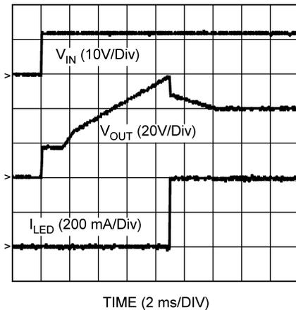
Figure 9. Power Up ( $I_{LED} = 0.2\text{ A}$ )
