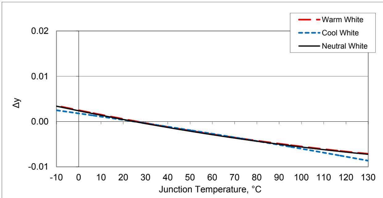
*Figure 5: Typical ccx Shift vs. Junction Temperature*
