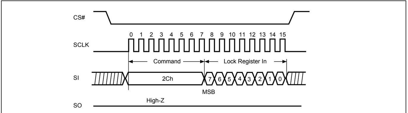
**Figure 81. Write Lock Register (WRLR) Sequence (STR-OPI Mode)**
