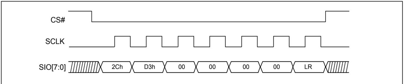
**Figure 82. Write Lock Register (WRLR) Sequence (DTR-OPI Mode)**
