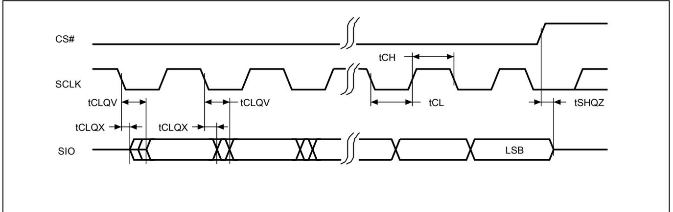
**Figure 4. Output Timing (DTR mode)**
