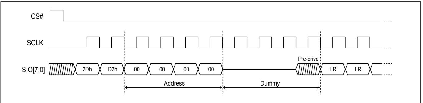
**Figure 79. Read Lock Register (RDLR) Sequence (DTR-OPI Mode)**
