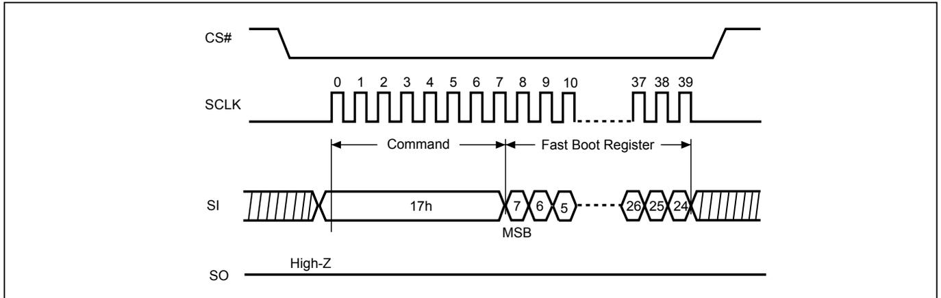
**Figure 56. Write Fast Boot Register (WRFBR) Sequence (STR-OPI Mode)**
