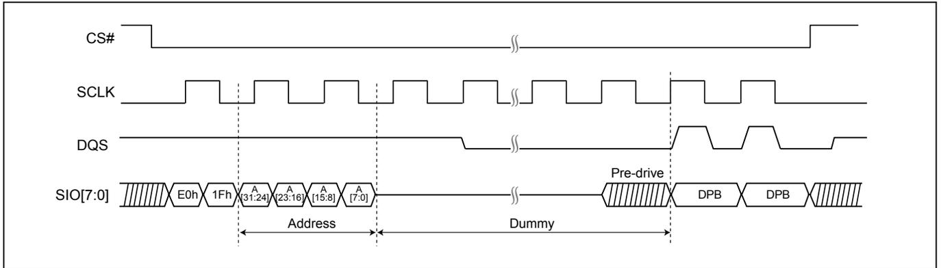
**Figure 94. Write DPB Register (WRDPB) Sequence**
