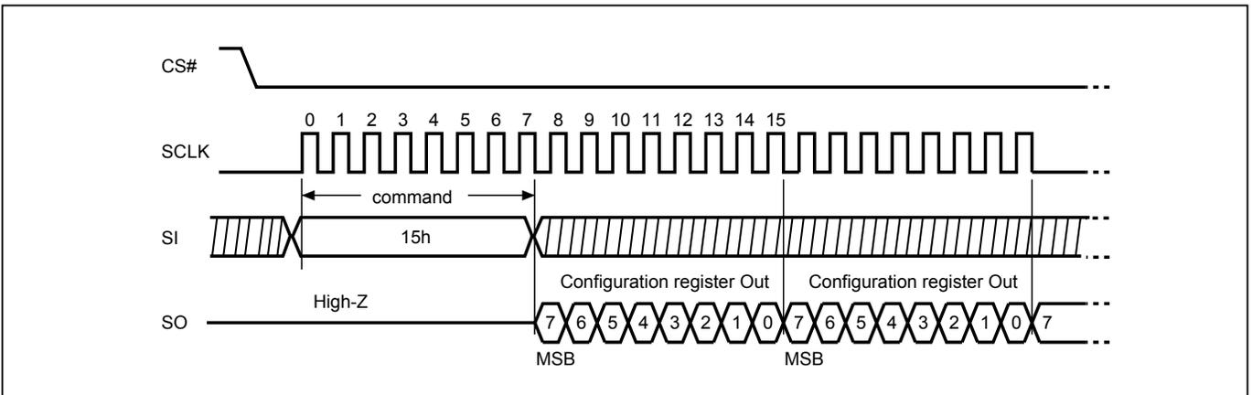
**Figure 20. Read Configuration Register (RDCR) (STR-OPI Mode)**
