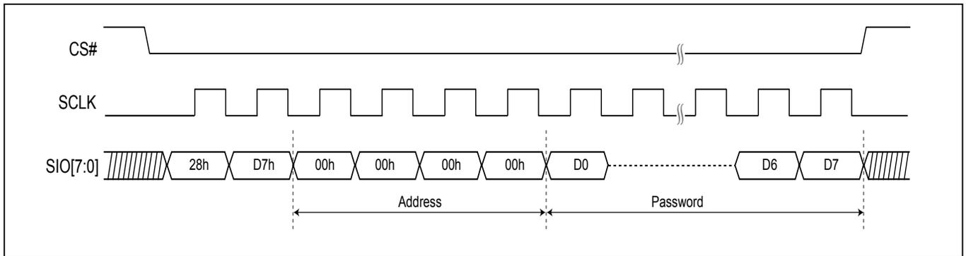
**Figure 103. Write Password Register (WRPASS) Sequence (DTR-OPI Mode)**
