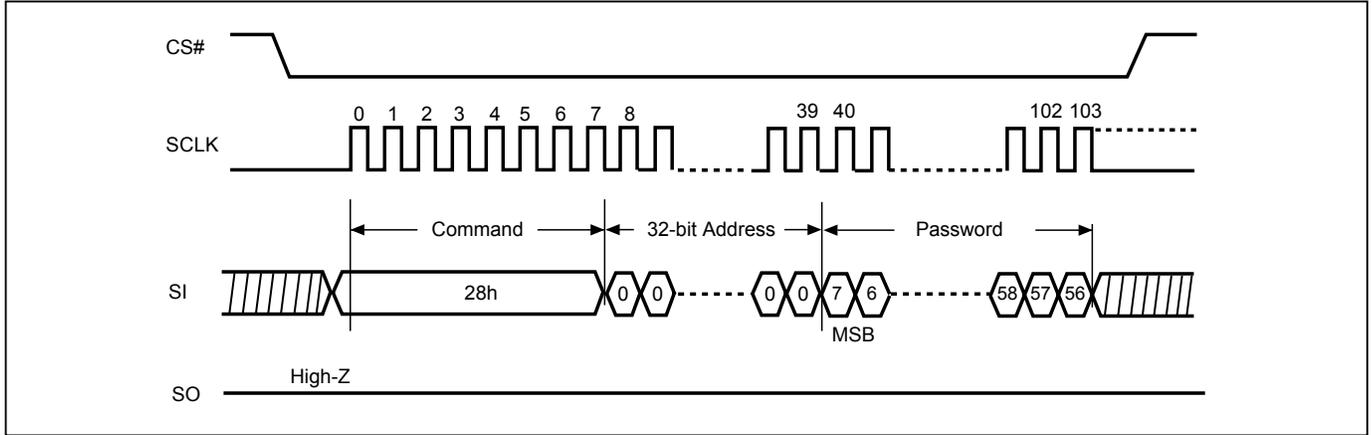
**Figure 102. Write Password Register (WRPASS) Sequence (STR-OPI Mode)**
