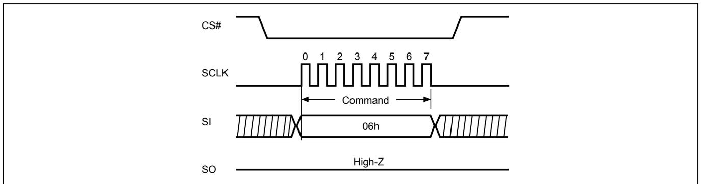
**Figure 6. Write Enable (WREN) Sequence (STR-OPI Mode)**
