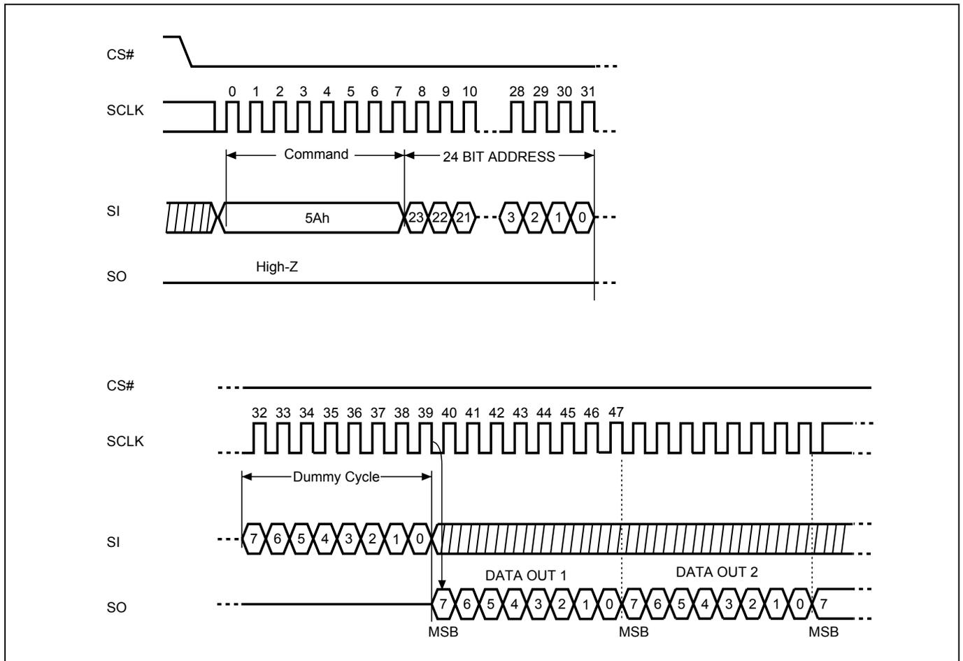
**Figure 115. Read Serial Flash Discoverable Parameter (RDSFDP) Sequence (STR-OPI Mode)**
