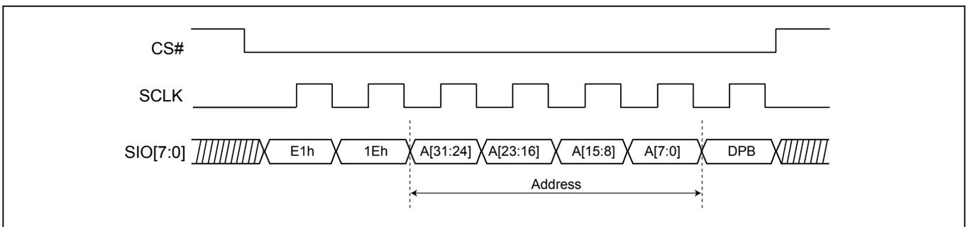
**Figure 97. Write DPB Register (WRDPB) Sequence (DTR-OPI Mode)**
