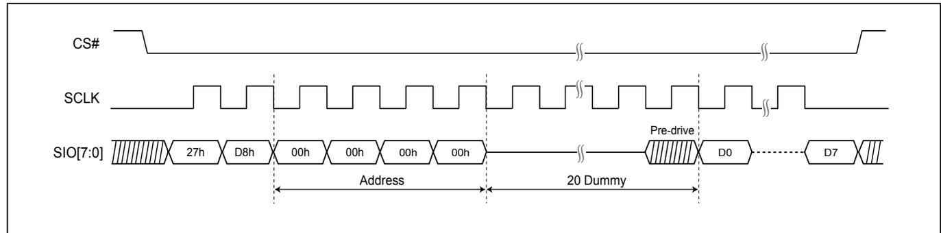
**Figure 100. Read Password Register (RDPASS) Sequence (DTR-OPI Mode)**
