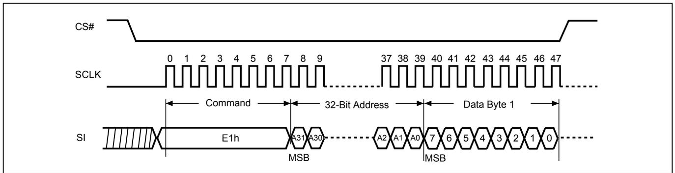
**Figure 95. Write DPB Register (WRDPB) Sequence (STR-OPI Mode)**
