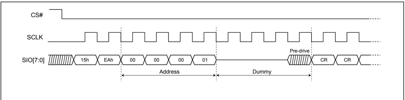
**Figure 21. Read Configuration Register (RDCR) (DTR-OPI Mode)**
