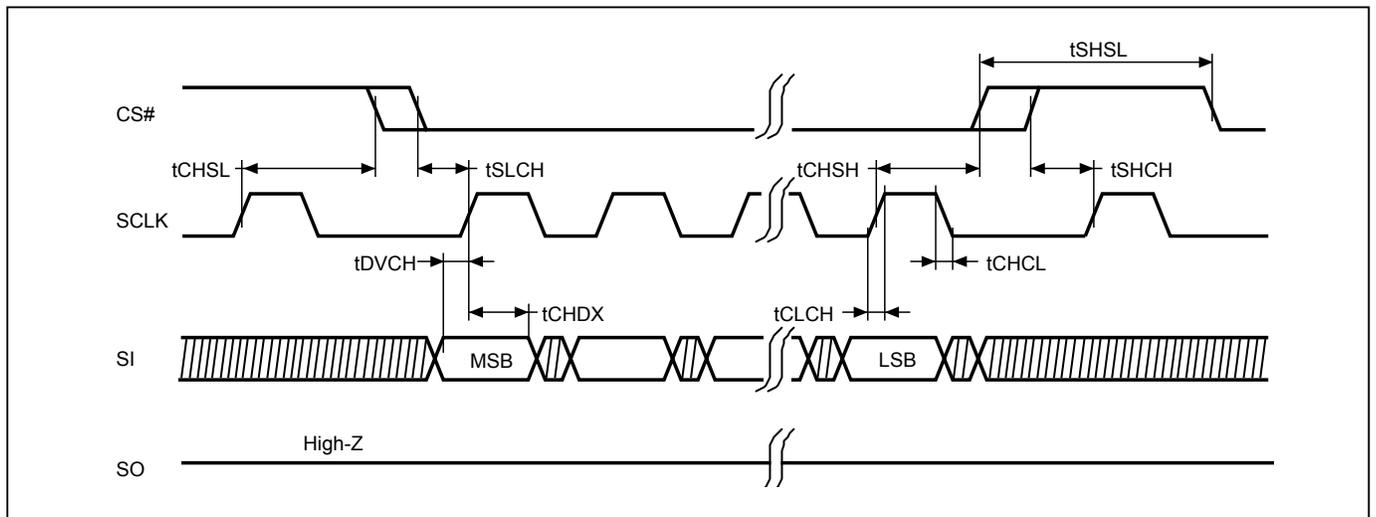
**Figure 2. Input Timing (DTR mode)**
