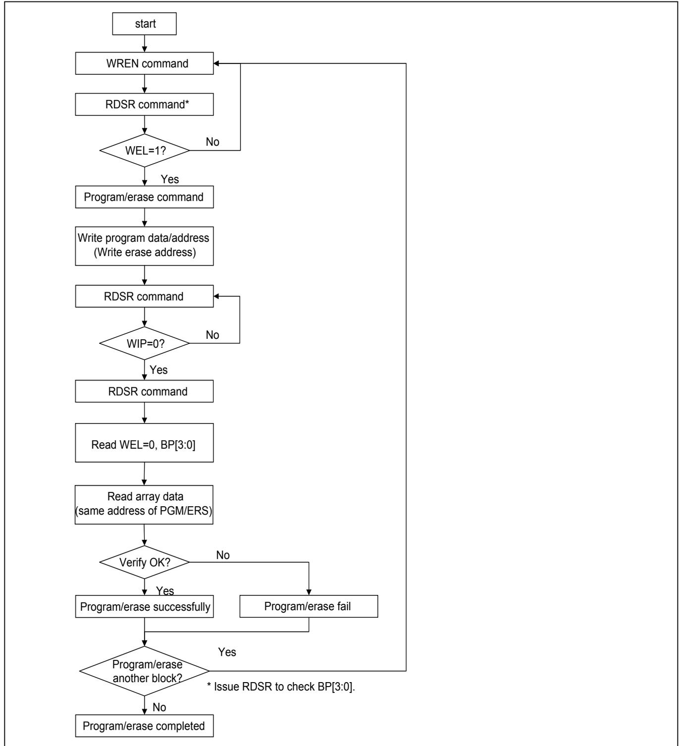
**Figure 18. Program/Erase flow without read array data (read P\_FAIL/E\_FAIL flag)**
